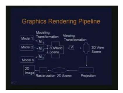
We have just elaborated that conversion we had from 3D scene to 2D image. I have a 3D scene which in fact is constructed using various models so I have model 1, 2 to model n.
