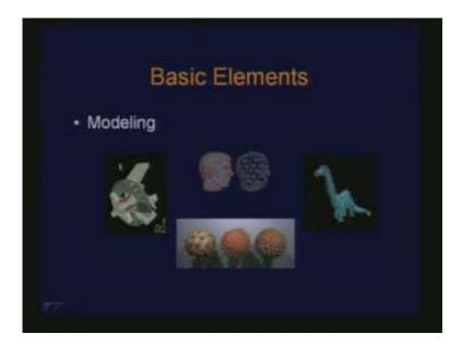
So we have some examples, this is some engineering part where we have collection of primitives there is a disk, there is some cylinder and there are other simple primitives. So it is an assembly of primitives together and then there are operations which could have union of them, subtraction of them and so on. This is one way of dealing with modeling, the assembling of primitives and operations of these primitives.
