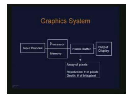
Now, if I want to see graphics more in terms as a system where I had the hardware which are used for the system I can see this as basically a collection of some input devices for instance keyboard, mouse or a unit which has the capacity of processing that is some memory unit which does this.
