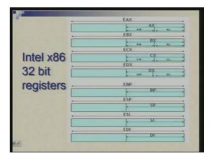
So here is a glimpse of register structure not all registers but I am showing all the major 32-bit registers of 8086. So they have a name like EAX, EBX, ECX, EDX this is one set where E and X are both there. Actually E stands for extension extended A register so actually extension has taken place in two stages so there were 8-bit architectures with
