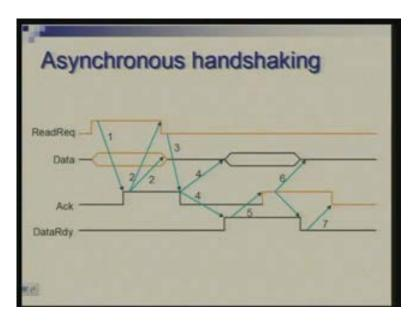
Just for your recollection here is the asynchronous handshaking protocol, one example we had seen and a synchronous protocol. So we are talking of a bus which is a 64-bit synchronous bus and frequency is 200 megahertz and we will see effect of varying the block size from 4 to 16. So now the protocol of the bus is as follows that it takes one clock cycle to send either data or address and we require two clock cycles between each bus operation.
