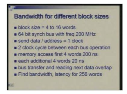
These are characteristics of the bus (Refer Slide Time: 06:15) and memory which is being accessed is capable of sending first 4 words within 200 nanoseconds and then each additional word requires 20 nanoseconds. So it has a mechanism within it that you do not need to repeat the whole transaction, it can actually get additional words within 20 nanoseconds.
