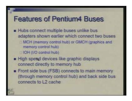
Here we have, what you would have noticed is that we have hubs rather than adapters. We talked of adapters trying to connect two different types of buses but hubs are somewhat more complex, we are connecting multiple buses.
