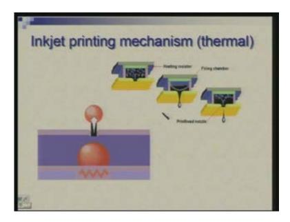
This is a thermal mechanism where the ink droplet is thrown out by a small, by very localized heating process. So here there is a heating register which gets which gets heated by electrical current and it is a very controlled heating, so by heating there is an expansion and the droplet goes out.
