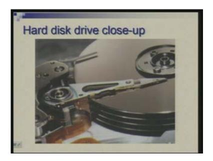
This is a real picture of a hard disk drive. Here you can see four platters, so there will be eight surfaces eight recording surfaces and this is the head, this is the head assembly and this is sorry this is the arm (Refer Slide Time: 35:37) and the head is actually close to the tip. So it is pivoted around this point so this head will move outside outwards or inwards, move from track to track.
