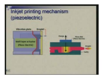
So this is ink cartridge where in this chamber there is ink (Refer Slide Time: 47:11) and here is a plate quartz plate which is piezoelectric and it can vibrate and by that vibration it can throw out a very tiny very fine finely controlled droplet of ink. So this vibration would be controlled by the electrical signal which it receives depending upon the information which is to be printed.
