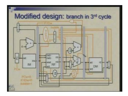
We are not making these pass through this register (Refer Slide Time: 7:42). The consequences of this are that the delay calculation which ultimately determines the clock period would undergo a change. Now you need to account for the multiplexer delay of this which we have ignored so far along with this adder and also with this ALU to look at the to consider the path delays.
