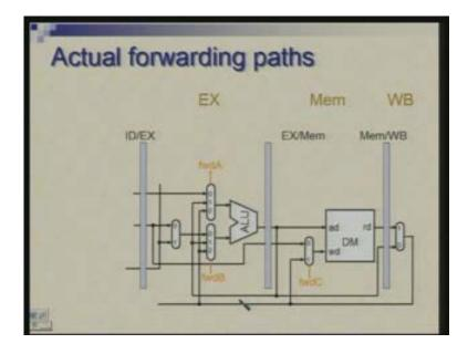
So, to improve things we had identified where we can have forwarding paths. So this diagram, for example, shows that you can have paths going from output of ALU through this inter stage register back to ALU or you could have output of the memory stage after this register and possibly after multiplexer going back to memory and also back too ALU.
