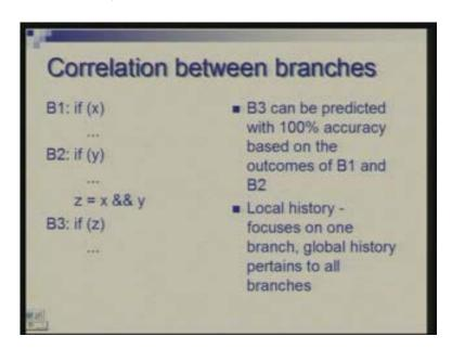
For example, look at this sequence on the left; you are testing some condition here, you are testing some other condition there then you are looking at something which is dependent on both these. So suppose z which is being tested here was x and y so now if you once you have gone through this and you have gone through this and the value of x and y have not changed in this course then it varies it to predict what z may be because
