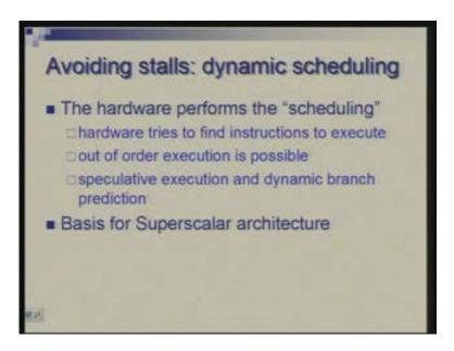
Instead of putting the instruction in the pipeline in the order in which they are occurring you try to analyze the instruction and push those instructions against the pipeline which can go through without causing any stalls so that is dynamic scheduling. What we are doing now, for example, when we are doing data forwarding we were trying to check the dependency between instructions and trying to take correct action.
