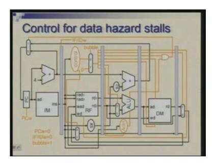
So now let us look at this design where you have datapath and control. It is same thing I might have re-rooted some wires just for the sake of clarity of the diagram. So now where is it how how do we introduce no operations and how do we prevent an instruction from moving forward.
