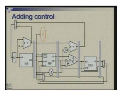
We will introduce a controller and try to generate control signals for all the components which require for example register files, multiplexers and so on.
