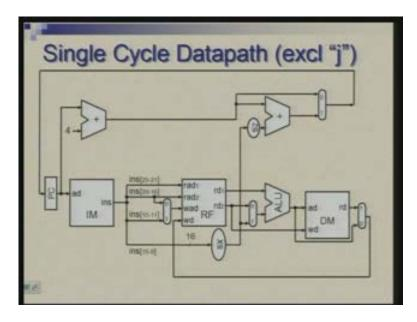
So you recall that we started with a single cycle datapath which was formed which was used as the basis for designing pipelined datapath. So just to simplify things we had omitted instruction j not because it is too complicated but just to reduce the size of the datapath so that it becomes easier for discussions.
