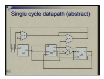
And another simplification we did was that we omitted some of the components like multiplexers and sign extenders and shifters so that again the number of components you see in the diagram is smaller and you can easily analyze and discuss. So the approach to the datapath design was basically to introduce the registers which would separate stages from one and another.
