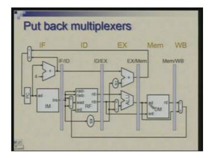
So notice here that if there is an R class instruction where memory stage is not being used then data is simply passing through and experiencing a delay of one cycle here. So essentially we are going through that cycle but not doing anything; idling through one cycle so that pipeline operates in a very homogenous and uniform fashion.
