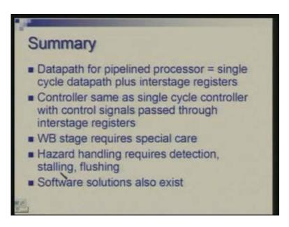
To summarize what we have learnt today; we completed the datapath design and datapath design which we have is nothing but the single cycle datapath design with interstage registers and we have to make sure that every line goes through write number of registers so that timing is correct so carefully one has to do that.
