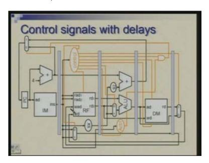
So all that I have done is I have extended these walls to separate control along with the data. So basically the signals which are effective within this cycle are going directly; the signals which are required here in the ALU stage is going through one register so basically you could see these two signals going to ALU control and going to this multiplexer.
