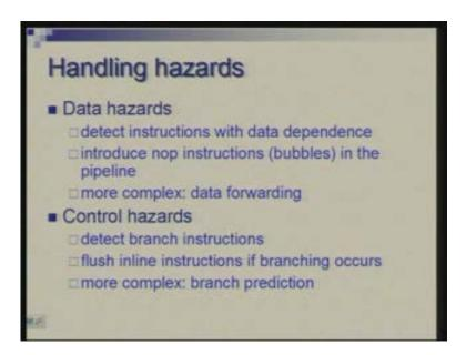
So, for data hazard the first thing is to detect instructions with dependence and you introduce suitable number of no op instructions. Sometimes a delay of two is required and sometimes a delay of one is required so in the pipeline where things are flowing moving smoothly you insert bubbles or no op instructions.
