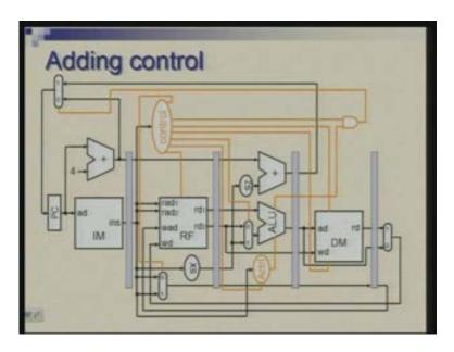
We still have not really seen that what is the influence of mixing of datapath from two different instructions. This is the address coming from this instruction which is here (Refer Slide Time: 21:55) and that is the address coming from instruction which is in that stage. But anyway the signal which is getting generated is found by ANDing a signal coming from controller and Z output of ALU. Finally we need one more for the multiplexer at the output end.
