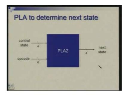
So here is the PLA which will implement these: 4 bits of control state and 6 bits of opcode to produce the next state which has 4 bits.
