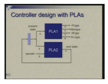
So here is the state register (Refer Slide Time: 8:18) it is a 4-bit register which contains the current control state and this drives both the PLAs; this PLA is generating the control
