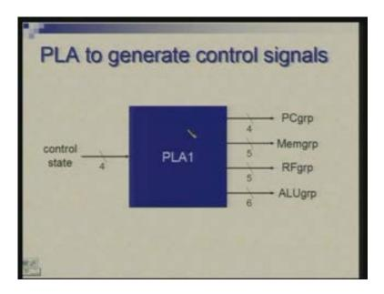
So this can be implemented by a PLA as we have discussed earlier for single cycle design. This PLA will have 4 input coming from the control state and four groups of control signals; group of 4, group of 5, another 5 and 6 so altogether twenty signals which go to the data path.
