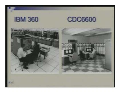
Two very popular systems: IBM 360 on the left and CDC 6600 on the right. Architecturally CDC 6600 was very significant. It introduced the idea of pipelining and some of the ideas of the modern day processors are actually traceable to this computer. I will discuss that when we go into more architectural details.
