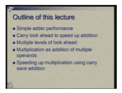
So, coming back to the simple adder circuit which we have discussed we had discussed how we do addition using paper and pencil and our attempt was to capture that in a simple circuit exactly the way we do it. That means we take the corresponding bits of 2 operands, perform the addition and let the carry go to the next stage.
