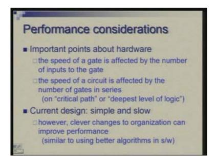
So, basically we should go down to how a gate behaves when input changes. So, at some point of time suppose the input changes, let me.... suppose we have AND gate and if you look at waveforms in time; suppose a is 1 and b is 0 up to some point when it changes to one then we expect that c would become 1 in response to this change but there would be some delay c is 0 at when at least 1 input is 0 so it is this delay which is attributed to the gate.
