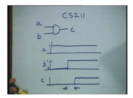
So, gate has transistors which switch from one state to the other state and it is that which takes time. Also, the gates are driving some load or some capacitance and that load has to be charged so the charging time of the capacitance is what dictates this delay. Without going much into details of this delay we assume that each gate has some inherent delay.
