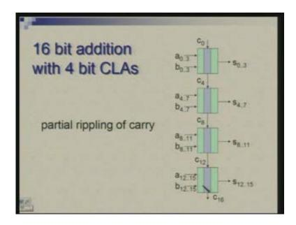
So remember that the carry comes out in 3 d time and sum comes out in 5 d times so let me let me write the time when the thing will come out at different points. so this is this comes at 5 d I will omit d; this (Refer Slide Time: 25:36) is coming out in time 3 and from this 3 to this output it will take another 2 so this just a minute this will take d plus 2 d 3 okay the carries which are coming out in this will be 3 plus 2 5 and 2 this will come out at after 7 d.
