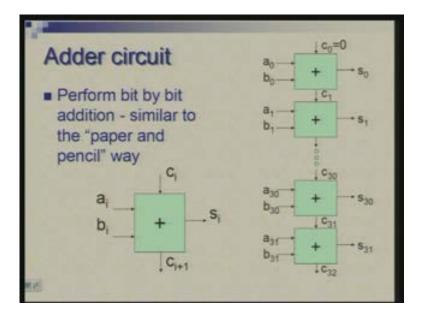
This is a circuit which adds two individual bits of the 2 operands and these 1-bit adders are cascaded or chained together to form adder of the right side. So, for example, if you are adding two 32-bit words then there are thirty two units which are put together like this. So in this you would notice that c 1 which is the carry out of the first unit is
