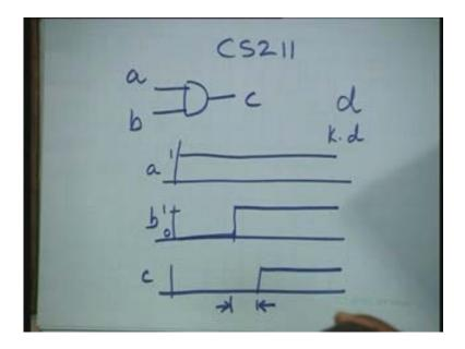
So, as I mentioned speed of the gate is affected by number of inputs to the gate and more strongly speed of circuit is affected by the number of gates in the series and there may be many paths you can trace in a circuit from input to output; the longest path the path which goes through the maximum number of gates in the chain is called critical path or the deepest level of logic.
