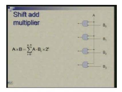
And the circuit for doing this can be easily built. First thing we are trying to do is multiplication with a 0 or 1 so it is effectively A is multiplied by one of the bits of B so here I am illustrating with a four bit situation. This AND gate actually represents an array of AND gates where each bit of A is ANDed with B 0. So, in [.....6:09] I am showing a single AND gate which is where we are taking a vector of bits A and a single bit B and output is a vector. So, strictly speaking I
