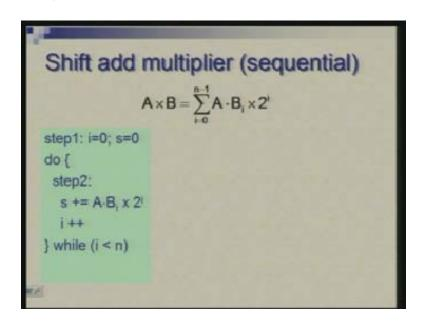
So what I am trying to indicate here is that there is an initialization step which is step one and step two which is repeated n times. Step two is both these assignments so actually what I imply is that all these both these are done together in the same clock cycle. So, for n-bit multiplication this would be done this loop will be done in n clock cycles; although I have written as two separate assignments but my intention is to do these two in hardware in a single cycle.
