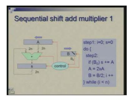
This has to work in conjunction with control which firstly takes care of this iteration count. The process has to be repeated several times so there it does the counting and it also times the operation of all other units. I am showing these red signals which are controlled signals; this is working under control of B 0.
