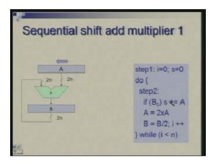
And to take care of this, A will be shifted left after A supplies, while A forms an input to this adder A will also make itself ready for the next cycle. So at the edge of the clock S plus A is a stored into this and 2A is stored into A. So these two events will happen concurrently with the edge of the clock.
