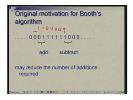
But of course in modern hardware each iteration takes one cycle whether you are doing addition or you are not doing addition so it is not considered as a mechanism to speed up things. But it gives us a mechanism to look at positive and negative numbers in a uniform manner and carry out signed multiplication directly.
