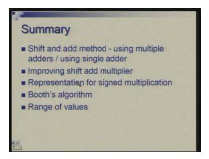
Although it is the original motivation was different which was to save the time it is a mechanism which allows signed numbers to multiply directly. And then we have also discussed range of the values and different MIPS instruction which look at the numbers differently as whether they detect the overflow or do not detect the overflow. I will stop with that.
