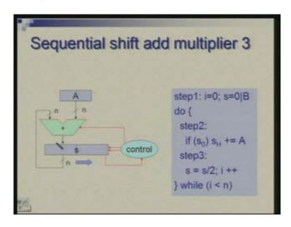
The initialization of S is different. We have 0 and B put together performing to n-bit word which is put in S and, yeah, here shifting of B is avoided there is no B register now so s become s by 2 which is a right shift and rest of it remains same. This is the final circuit which we will I will leave at. It requires one 2 n-bit registers one 1-bit register and a single n-bit adder.
