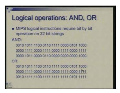
So the circuit for doing this very simple; there is no relationship between what you are doing for bit i and what you are doing for bit j. So, for each bit position you have an AND gate so ith AND gate AND a i and b i to give you s i. Similarly, ith OR gate out of thirty two OR gates OR a i and b i gives you s i which is OR of these two.
