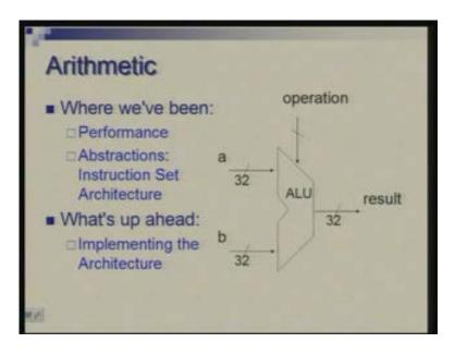
So essentially what we are aiming at is designing something like this an ALU which typically works on two operands; in our case for MIPS processor they will be 32-bit operands and produces a result under control of some signals which are determined from the instruction. So depending upon which instruction you are trying to execute this unit will perform some operation, it might perform addition, subtraction, multiplication, division or do some comparison or do some logical operation.
