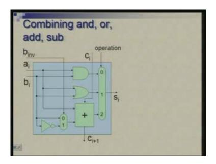
So this multiplexer has now three inputs (Refer Slide Time: 41:18) which I have labeled as 0 1 and 2 and depending upon a control input which is labeled as an operation either you will select this or you will select this or select this. So the input a i and b i are spread out to all these three components: to AND circuit, to OR circuit and to this adder cum subtractor.
