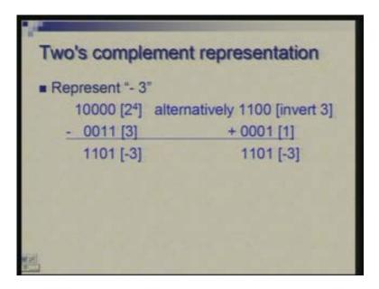
You subtract a binary number from all 1's basically each bit will get flipped and then you are adding a 1 later on. So this just shows the relationship between two ways of looking at it.
