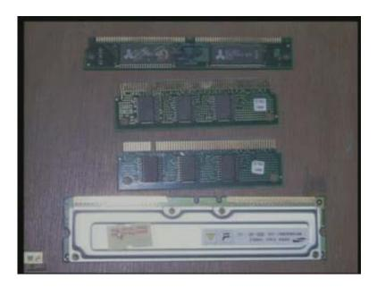
This is a memory module, this is in a package form, this is open another one, these are individual memory chips and all these put together form a memory module and several of these form the complete memory system.
