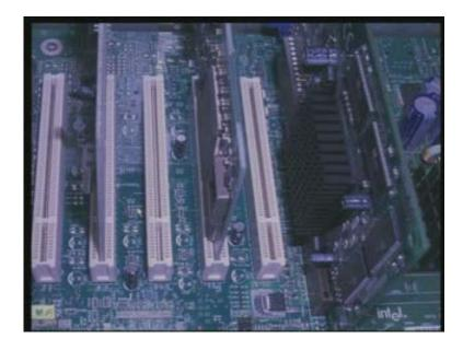
These are slots where you can plug in input output controllers, these are PCI slots, PCI is the name of the bus through which various cards are connected, various controllers are connected to the computer.
