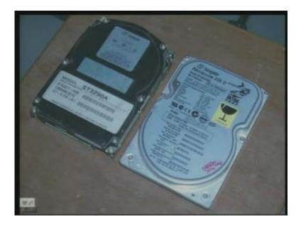
This is a Seagate hard disk drive shown from two sides. This part is the disk controller this is just a casing; you are not actually seeing the medium on which the recording is done that is inside. This is the controller circuit you can see closely (Refer Slide Time: 20:25).
