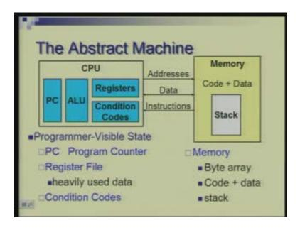
So, what is the basic principle on which a computer works is captured here that you have a memory which contains code or program in machine language and the data on which it is supposed to operate. Of course there have to be means to bring in data on which one has to operate and after computations are done take the results out. And, often memory contains a specialized structure called stack which is used to create functions or routine hierarchy of the program abstractions.
