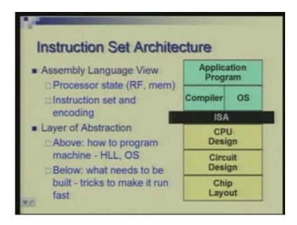
This is the typical view of where we place instruction set architecture in between software and hardware. At the top you have application programs which are able to run on a processor with the help of some system software. For example, compilers require translating these high level programs to machine code and OS is required to manage the resources and make it possible to compile, load and execute programs.
