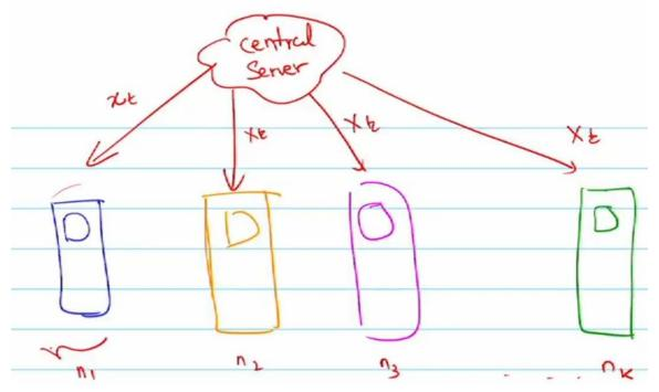
So, what this central server would do is, in some communication round t, it would basically broadcast its weight  $(x_t)$  to these edge devices. So, this x t is broadcasted.
