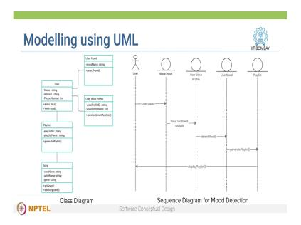
There are other models like the unified modelling language diagrams or UML diagrams, and these can help us represent the software design via multiple views and at a greater level of detail. We will learn more about modelling using these UML diagrams in the next video.
