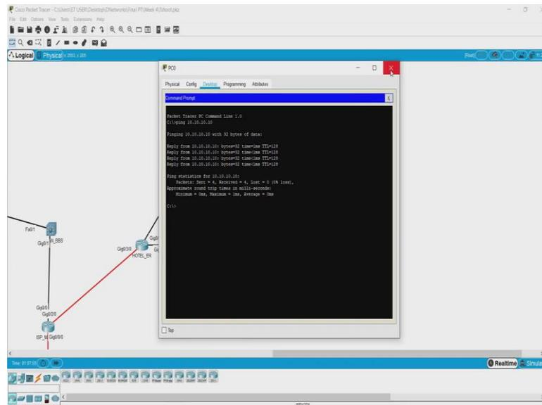
So, how we can do that? Go to the desktop and go here and again type ping 10.10.10.10 yes. So, we are successfully connected to the IoT server ok. So, now, that is not the issue then. So, let us go on to the server and check if we are able to access the smart devices from there. Now as we saw the connectivity is fine. So, one of the issues could also be thus service level issue on the application that is the IoT service is it running on the server or not.
