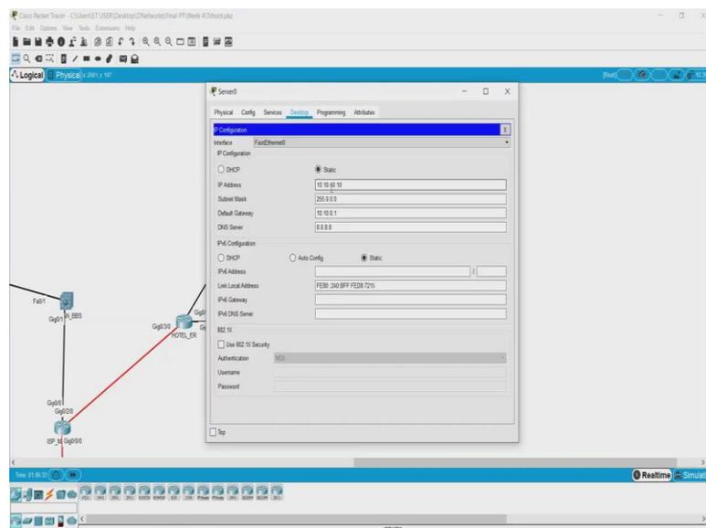
So, this is our server and the IP address of this service 10.10.10.10. Now do not get confused about this IP address and the IP address we saw in the college network these both are what? These are yes these are private IP addresses and two different networks can actually use the same series of IP addresses if they are not connected on the same router because one router cannot have the same series of network running on two of its interfaces.
