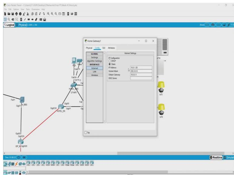
So, what is the scenario here? So, let us open the home gateway here look at the configuration tab and check the IP addresses. So, it is network IP is 10.0.1.20 and local area is 192.168.25.1. So, we have a Smartphone here. So, we can connect we can see if the connectivity of the gateway and the Smartphone is working or not.
