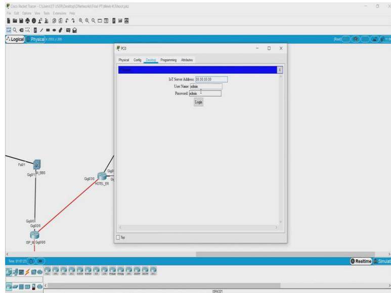
So, let us go to the PC and what we will try to do is, go to the IoT monitor and type the IP address 10.10.10.10. So, admin is default login that you have and login, but still you cannot see any IoT devices over here ok.
