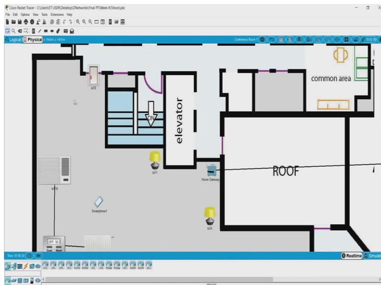
What you can see is there is a door here which is locked, this red light shows locked. So, we can physically unlock this door and open it. So, it is the way you do it in packet tracer is you press alt and click on the red link, see it turned green and you can unlock it, but this is not the way you want to solve the problem. So, what we want to do is, we want to see why is the communication not happening.
