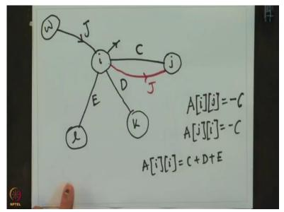
And if I want to add a conductance, then to A[i][i], the value has to be added, see this, and also to A[j][j] because the conductance is connected to and the treatment is symmetrical. And
