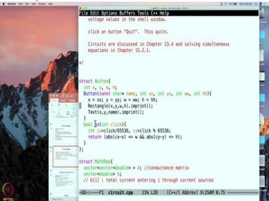
So, this is our class for representing buttons. So, it has data members x, y, w and h. And these data members are going to keep track of the centre of the button. So, that is the x y will be the centre of the button. And w will be the width, h will be the height. Now here is the constructor which is going to be called with the title that should appear and then the x, y, w and h are passed as parameters. So these parameters are stored into the data members and
