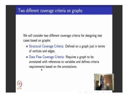
So, moving on we will look at two kinds of coverage criteria related to graphs. The first coverage criteria that we will be looking at is what is called structural coverage criteria where we will define coverage criteria purely based on the vertices and edges in the graph right.
