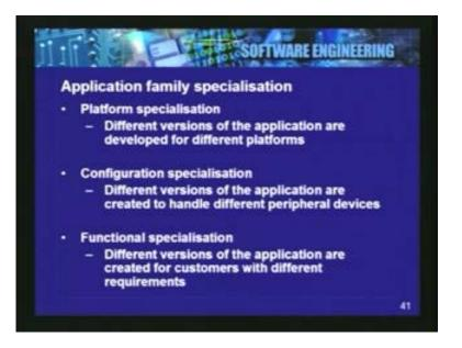
Different kinds of specialization can be done here. Platform specification can be done so different versions of the application are developed for different platforms. The common strategy that are adopted there is that there is a platform specific portion that is abstracted out and then there is a platform independent portion and for the platform specific portions different platform modules may have to be developed.
