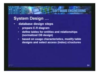
In fact a simple thumb rule could be that for every entity we have one table or one file and for every relationship also we have one file. So based on this we can prepare the table design; table design is what we do for relational database packages. So here are some of the tables that we will define.
