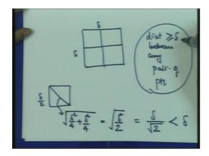
So, I have this square of size delta. And I know that, if I have any point in this square. Then, no other point is within a circle of radius; which means given any two points, the distance is at least delta between any pair. So, the distance between any pair of points in this square, is at least delta. How many points can I put in inside this square. Well, here is the trick, what you do is divide this into four parts. These will be our holes, you have to see where the pigeons are.
