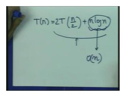
Your recurrence would look like T n equals T n by 2. Well, 2 T n by 2 plus n log n, because this sorting will dominate. Once, we sort we can go over them in linear time. But, this sorting will dominate and take n log n time. This the solution to this recurrence is still not n long n, the solution you can check that the time to find what the solution recurrence is n log n square and it is not n log, we would like to be positive.
