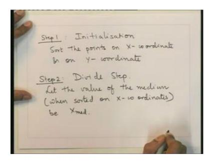
The first step is initialization, it is initialization. And here we sort the points on x coordinates and on y coordinate. So, given the set of input points we form two lists. So, we have two arrays. One array which will store the points in increasing order of x coordinates. The other array will store the points in increasing order of y coordinates. And this will be the input to the procedure.
