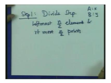
Step 1 is the divide step, this is the divide step. Well, I have the point sorted on x coordinates. So, I can find the left most, so since points are sorted on x coordinates, find the left most n by 2 elements and right most n by 2 points, these are points. This sort this give you the two points, the two sets. Now, I need to do this even for the points sorted on y coordinates. So, I have two arrays remember.
