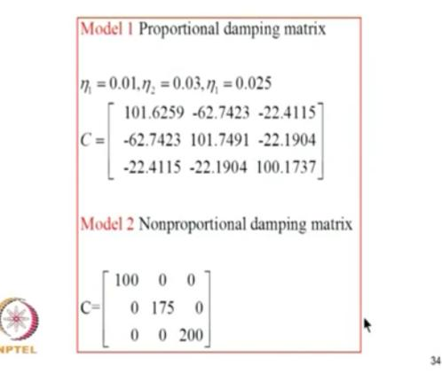
because the simple problem we will consider two alternative models, one is proportional damping matrix with damping ratio specified for the 3 modes to be 0.01, 0.03 and 0.025, this is one model, and associated with this, this will be the C matrix which we can compute following the procedure that I outlined.
