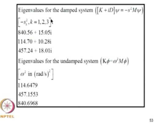
Now you can look at now the eigenvalues for the damped system I get this, you can see here the real parts are again close to the un-damped square of the natural frequencies, but they are slightly different because of influence of damping, okay, so now if we can quickly summarize
