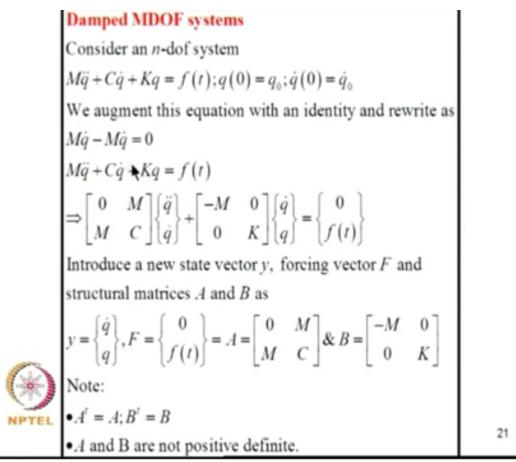
if you go back when we wrote this additional equation the way we converted this N second order equations to 2, and first order equation there are other ways of doing it, I will come to that later, this way of doing ensures that these coefficient matrices are symmetric, okay, so that is helpful you know to consider orthogonality relation, so now since the A and B are symmetric this equation can be written in this form, so this is equation 5.
