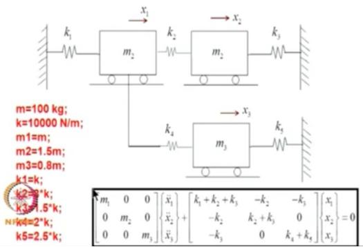
through a numerical illustration so let's consider 3 degree freedom system, configured as shown here and these are the numerical values and if I write the equation of motion for this system I get for the un-damped free vibration this is the equation, so we can quickly do the calculations
