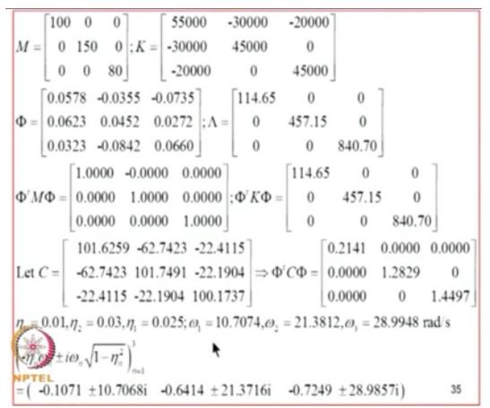
this is a mass, this is stiffness, after we insert the numerical values, we can show that the undamped normal modes this is the model matrix, and this is the matrix of eigenvalues. You can see that Phi transpose M Phi is the identity matrix, Phi transpose K Phi is the lambda matrix which is same as this, squares of the eigenvalues or the eigenvalues themselves squares of the natural frequencies.
