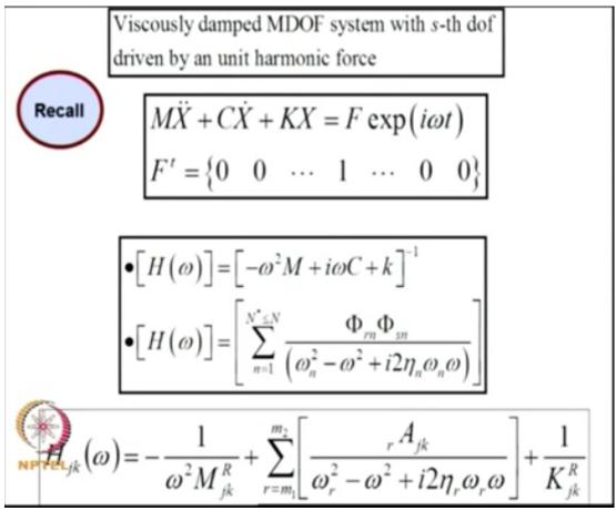
So we discussed the problem of finding frequency response function for viscously damped multi degree freedom system, so if we drive the S degree of freedom by a unit harmonic force we have shown in the previous lecture that the matrix of frequency response functions can be evaluated either directly by inverting this matrix, the so called dynamic stiffness matrix or we can evaluate in terms of un-damped normal modes and we get this as a summation.
