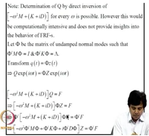
the note is that determination of Q by direct inversion of dynamic stiffness matrix for every omega is possible, however this would be computationally intensive and does not provide insights into the behavior of a frequency response, it is characterless description.
