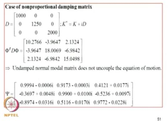
so again I consider D to be this and K star is K + ID, quickly we can verify phi transfer D phi is not diagonal, so it is not a classically damped system, so now I can do a complex eigenvalue analysis and I get this as Sai matrix, so we can verify Sai transpose M Sai is this, Sai transpose K Sai is this, these are diagonal but Sai transpose M Sai is not identity this is not, this is again diagonal but diagonal entries are not the eigenvalues.
