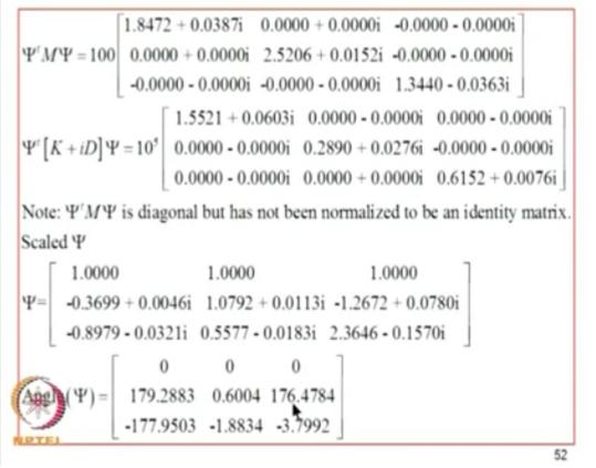
So I will scale now the eigenvector so that the first element is 1, I get this as a scale Sai matrix and if I now compute the angle of this you see now I get phase difference of about 2 degrees and less than 1 degree here and 0.6 degrees and 1.8 degrees and about 4 degrees and here, so this is a manifestation of the role played by damping on eigenvectors.
