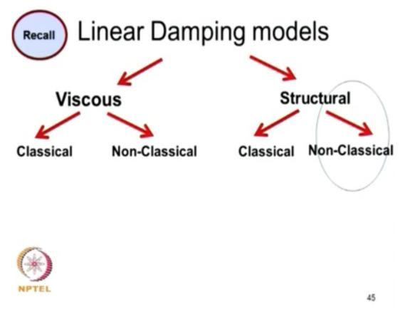
Now I have now discussed non-classical viscous damping system, now I will extend this formulation to structural damping with non-classical damping, so we consider the N degree of freedom system, this is the structural damping term which is the complex part of the stiffness
