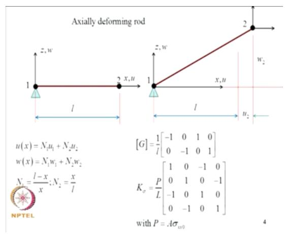
Using this and combining with the geometric stiffness matrix that we derived for Euler-Bernoulli beam we formulated the 2 1 dimensional beam element, and that beam element to
