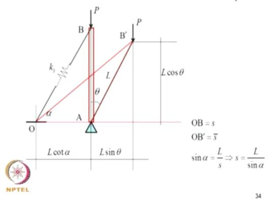
Now let's come to the asymmetric structure, suppose this is the bar which is supported on spring like this at some time, at some snapshot it would have deform like this, and we have to set up the expression for the total potential, so we have to find out the amount of stretch in the spring and the work done by gravity, so I mean the moment through this distance, so if initial length is OB is S, and OB bar is S bar, the energy stored in the spring is 1/2 K S bar - S whole square,
