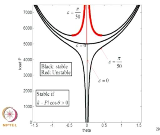
I plot this, this is how it will look like, suppose epsilon = 0, this Y axis I have the load and on X axis I have theta, so as a load increases the load deflection path rises along this curve, and once the P critical value is reached the theta = 0 solution becomes unstable, the red lines are unstable, and black lines are stable, where in the stable branch bifurcation to do other branches like a bowl as shown here, okay.
