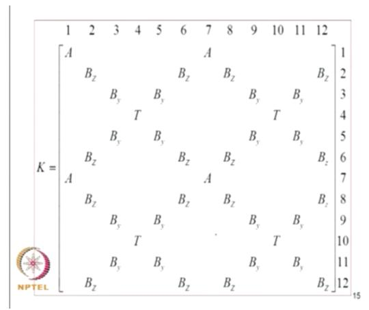
Now we can simply assemble the matrix including these effects, so if you name the degree of freedom as shown here 2 nodes and this is a nomenclature of degrees of freedom, the field variables are U, V, W and theta, if we do that, if you recall this we already seen and these for example 1 1 element will be due to axial deformation. Similarly 7 1 will be due to, see for example 7 and 1, 1 and 7 are axial deformation, etcetera, etcetera, so this will get filled up, and
