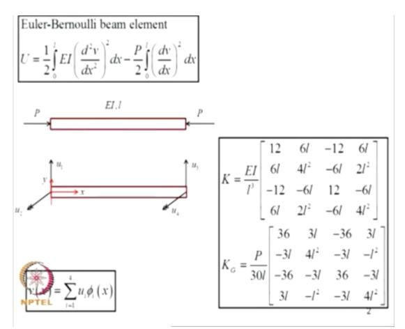
last class we derived the geometric stiffness matrix for an Euler-Bernoulli beam and this is the total potential and we use this as a trial function, and this is the geometric stiffness matrix that we derived.
