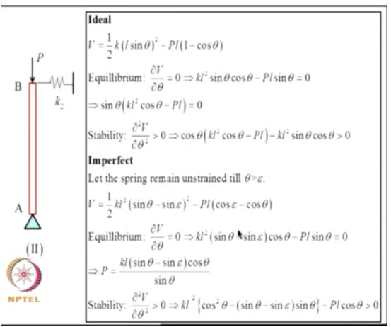
Now let us consider the second configuration where the bar is supported on a spring as shown here, again the potential is given by 1/2 KL sine theta whole square - PL 1 - cos theta, for equilibrium this is a condition this is in fact is a load deflection diagram, there are two equilibrium path sine theta = 0 and this equal to 0, now for stability this condition must be satisfied, okay, this is straightforward derivation.
