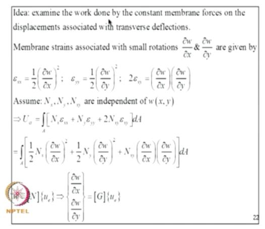
forces on the displacements associated with transverse deflections, so membrane strains associated with small rotations you know these are given by this, okay, this is extract from the appropriate strain displacement relations, I am retaining only the relevant nonlinear terms, the linear terms lead to equivalent nodal forces associated with the initial stress that I am not discussing.
