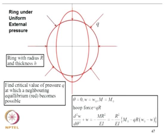
Now if the beam ring is now loaded by a uniform force field as shown here, can it assume a neighboring equilibrium state, for example the I've shown in this elliptical curve, this is the ring in the un-deformed configuration, Q is the load which is axisymmetric constant external compressive load, so how you leaving deform.
