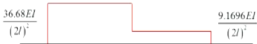
Axial thrust diagram on the verge of buckling
