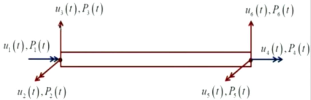
2-noded element with 3 dofs per node
