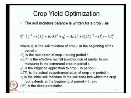
First, we will start with an optimization problem, where a known amount of water has to be supplied to a particular crop across time periods t. Now, this is the soil moisture balance, this is at the beginning of the time period t plus 1, the root depth is D t plus 1 for the crop c.
