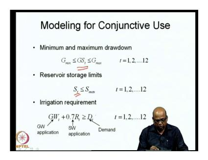
Then we put all other conditions that ever ground water storage must be within this two limits; the surface water storage must be less than or equal to S max. And then we put the condition that whatever you apply at the irrigated area, namely the ground water pumping, ground water application plus the surface water application must be greater than or equal to the demand itself D t.
