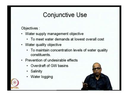
Now, for the systems models, when we are looking at the conjunctive use of surface and ground waters, we may have several objectives; for example, the first level of objective that we may want to fabulate is to meet the water demands at lowest overall cost. So, you want to create a surface water infrastructure, and you want to create a ground water infrastructure, to meet a certain demand pattern; and this infrastructure that we create
