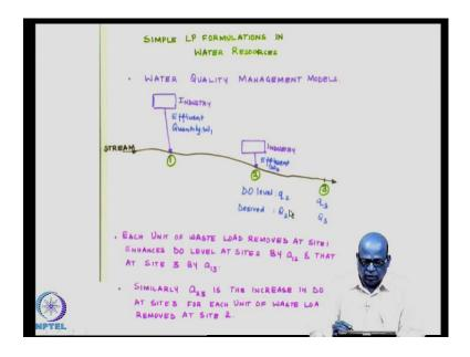
It is a simple problem of water quality where we are interested in maintaining water quality at these 2 check points, point number 2 and point number 3. This is the stream which receives a effluence from 2 industries, industry 1 here and industry 2 here with the effluent quantity of w1 and effluent quantity of w2 at location 2. If you do not provide
