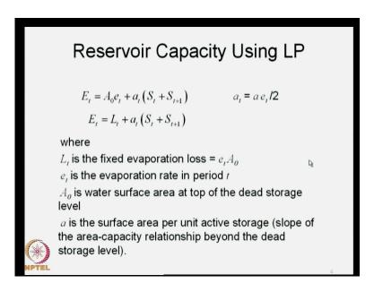
What is a t? a t we defined as, a into e t by 2, and a is the slope of a area capacity relationship beyond the dead storage, e t is the rate of evaporation therefore, you can get a t, because e t changes from one time period to time period. Although, a remains constant, a t changes from one time period to time period.
