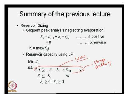
So, if you recall the sequent peak algorithm, we write it as K t is equal to K t minus 1 plus R t minus Q t; R t minus Q t in any given time period t. In fact, indicates the deficit that occurs during that time period, Q t is the inflow, R t is the demand or the release the from the reservoir, which we set it to equal to demand.
