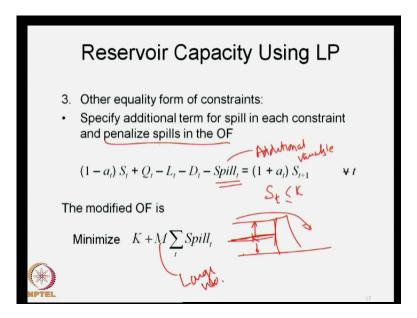
We also have another way of doing it, we can specify spill explicitly; this is the overflow. So, typically what happens is as I said your reservoir capacity comes up to K and then additional amount, we put it as spill. So, we are putting another variable (()) spill as on additional variable.
