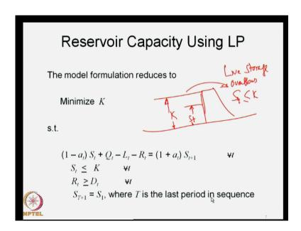
Now, let us see, how we state the problem and therefore, we state the problem as minimize K, which means we are looking at that particular storage capacity K, minimum storage capacity K, subject to the storage continuity equation, which account for the evaporation losses written for all time periods t, S t is less than or equal to K, because the storage must be less than or equal to the capacity.
