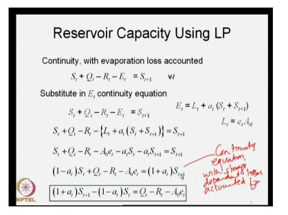
So, the storage continuity equation was S t plus Q t; that is the initial storage plus the inflow minus the release minus the total losses E t is equal to the end of the period storage S t plus 1; the evaporation loss E t we just wrote it as L t, which is e t into A naught plus a t, which has A naught e t by 2 into S t plus S t plus 1. So, this is what we substitute here.
