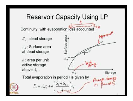
So, let us look at, how we account for evaporation as storage dependent losses? Now this is the area capacity relationship, this is storage on the x axis, surface area on the y axis, this is water surface area or water spread area, typically we will have this curve like this.
