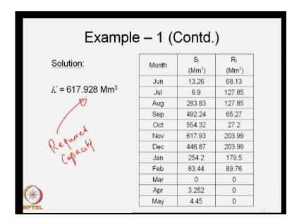
So, when you solve this, you get the solution like this, S t and R t and the associated K value. So, this is the storage capacity, required capacity.
