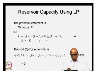
So, we will write this problem in using this formulation of the constraints as minimize K; that will remain as it is, this is the objective function, subject to 1 minus a t plus Q t minus L t minus D t greater than or equal to 1 plus a t into S t plus 1.So, instead of equality constraint here, I making it as greater than or equal to and S t less than or equal to K.
