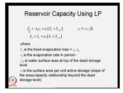
So, we will write this as E t is equal to A naught e t; and then, I will introduce for a into e t divided by 2; a e t by 2, I call it as a t some constant a t, which in this from time period to time period, because e t changes from time period to time period. So, I will write it as a t is equal to a into e t by 2; and therefore, I write E t as A naught e t plus a t into S t plus S t plus 1.
