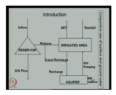
Then, we look at the conjunctive use of surface and ground water. You typically have a reservoir from where you have a canal network and then, you have irrigated area. From the irrigated area, the evapo transpiration takes place. There is the rainfall that is feeding into the irrigated area. Part of it also comes as recharge. What you are letting out through the reservoir can also contribute through seepage as canal recharge and then this canal recharge goes to aquifer.
