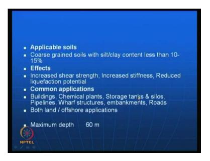
In a simple form it is a penetration. Then, there is a vibration here. Compaction has been done in the horizontal direction, then you also backfill the material. Say for example, you
