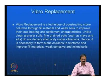
So, that is about Vibro-Compaction. What about Vibro Replacement? The Vibro Replacement is a technique of constructing stone columns, through the fill material and the weak soil to improve the load bearing capacity and settlement characteristics. Like
