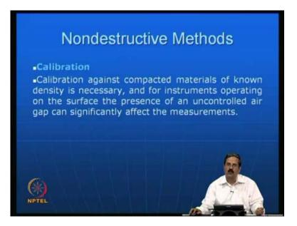
As I just mentioned calibration is important here and calibration is against the compacted materials of known density and for instruments operating on the surface the presence of an uncontrolled air gap can be significantly affect the measurements. So, one should be very careful with the air gaps presence of air gaps and all that because you know through the air you know there could be misleading results one should be very careful there.
