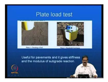
And nowadays what is called see actually plate load test that we studied is also an important approach to measure the say for example, plate load test we use to calculate the modulus of sub grade reaction in the case of pavements like k value you get.
