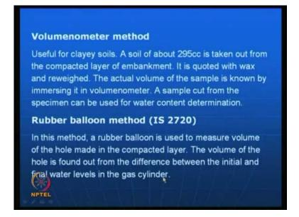
Then you have what is called rubber-balloon method. In this method, a rubber-balloon is used to measure volume of the hole in the compacted layer. The volume of the hole is found out from the difference between initial and final water levels in the gas cylinder.
