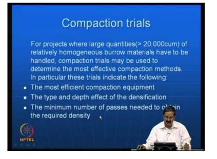
Sometimes like in a big project the advantage would be that you better do compaction trials because what happens going by certain specification is one thing, but try to come out with project based specifications like you have a big area somebody have some 10,000 crores project in a for an embankment or a this thing is better that you have a specifications based on the material available there and try to understand the soil behavior of the materials.
