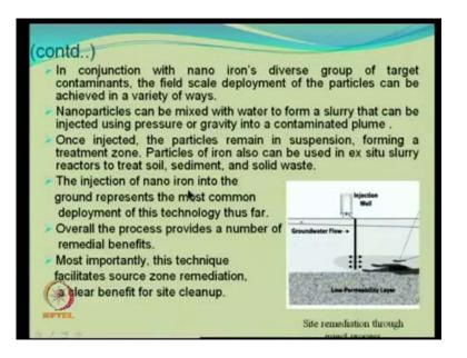
So, in conjunction with nano iron's diverse group of target contaminats, the field scale of may deployment of the particles can be achieved by varieties of ways. Nanoparticles were mixed with water to form a slurry that can be injected using pressure or gravity into a contaminated plume.
