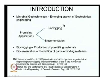
And In this talk, I would be talking about the applications as I just mentioned you have this microbial geotechnology something that has come that is emerging in the recent times and I would be talking about two applications namely bioclogging and biocementation.
