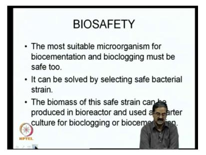
So very important thing that I mentioned earlier was that the biosafety the most suitable microorganism for biocementation bioclogging must be safe like you are trying to use it it should be safe it can be soiled by selecting a safe bacterial strain. The biomass of this
