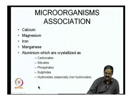
So you have couple of materials that are required here say they are quite helpful in the in the formation of cementation if you have calcium, magnesium ,iron, manganese and aluminum which are crystallized as carbonates carbonates, silicates ,phosphates and sulphides and hydroxides definitely the there is a possibility that you get good cementation.
