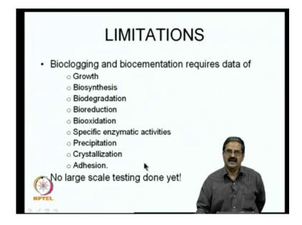
Ah bioclogging and biocementation require the data of growth of the bacteria the biosynthesis, the mechanism of biosynthesis, the biodegradation ,the bioreduction biooxidation specific enzymatic activities precipitation crystallization a,dhesion so these are all some important inputs like see when you add bacteria into soil you must be able to understand what is the growth of bacteria and how is it going to react with the soil.
