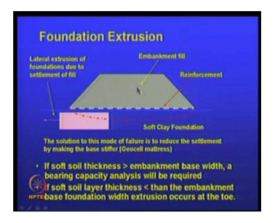
Now, what is this foundation extrusion? What it means is that see, you have put a reinforcement is there everything is fine, but then the possibility is that if the if the soft soil thickness is more than the thick you know, embankment base width.
