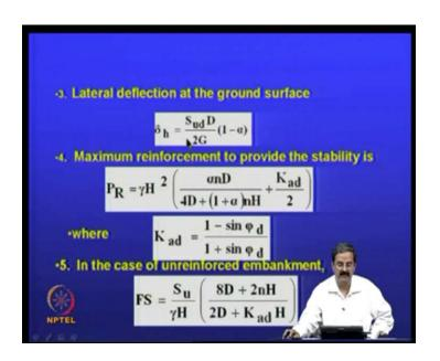
And what is a displacement also we have seen is simply that I just mentioned S ud by 2 G, we have already seen that, but how is that alpha is coming into picture, alpha is that when inward shear stress equal to outward shear stress alpha is 0, and if you have alpha term, how does it influence; because alpha is another important variable and that what we see; that is one term.
