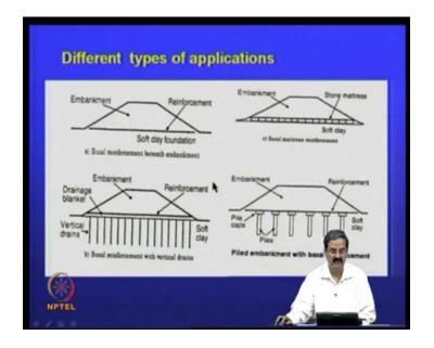
So, what are the applications? There are too many here, actually, wherever there are soft soils, it is well established, and you have an embankment here, you put a reinforcement like this, it is called Basal reinforcement beneath embankment.
