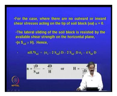
And that can be, this understanding can be used to calculate what is called like this, say for the case where there no outward or inward shear stresses, we can say that the alpha is 0, you know, there is one case that it is just under equilibrium.
