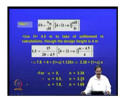
So, for that step one, like the factor of safety of one, you know, factor of safety using this reinforcement is this equation; sometimes, though I have the and a problem we know that the it is a 4 meter is the height of the embankment, you can even take a 4.5 in calculations to be on the safe side, that is one thing.
