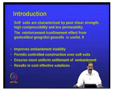
We know that soft soils are characterized by poor shear strength, high compressibility and low permeability, and if we are able to use a reinforcement effect when you have a geosynthetics or you know, we have different types of materials that we studied, when you have a geotextile or a geogrid or a geocell, they introduce, you know, reinforcement function; actually, it is also called pseudo confining pressure.
