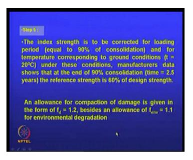
So, the the index strength is to be corrected for loading period, which is equal to 90 percent of the consolidation, and for temperature corresponding to ground conditions; assume that it is temperature 20 degrees.
