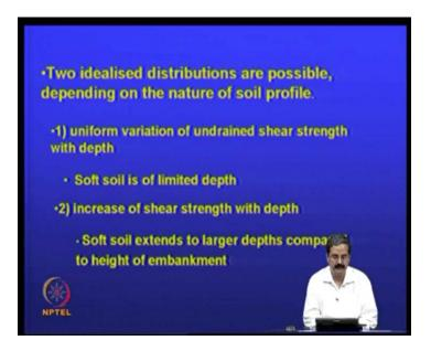
Another point that I would like to highlight is that when there is a soft soil, there are a they how does shear strength vary with depth? Actually, if the soft soil is a two shallow, one can assume uniform variation of undrained shear strength with depth.
