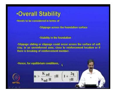
That is have the one one more thing is that slippage across the foundation surface, you know, in fact, it should not the see as I said, it it should not slip through the reinforcement, and then it should not also slip through the soft soil.So, we have used a factor alpha, D s when it is trying to slip through the across the reinforcement, but when you want to say across the foundation surface, foundation has what is called the shear strength of S ud.
