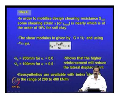
So, how does it really matter in in terms of the displacement? So, in order to mobilize design shear resistance S ud, some shearing strains is nearly is required, which is actually, why I just, what is a basis of this 10 percent, like you know, you see a you do, what is that Vane shear test right? Vane shear test if you do, it just you know, you do the Vane shear testing it give some number which is ultimate shear strength.
