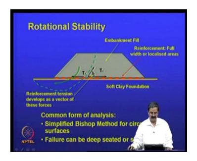
And then, so what is this rotational stability? Like, you know I was just trying to... The example is that, say for example, this is that failure surface right; if this is a failure surface and the driving forces are like this, and then the resisting forces are in the opposite direction. So, if this driving force... This is the embankment material and this is reinforcement.
