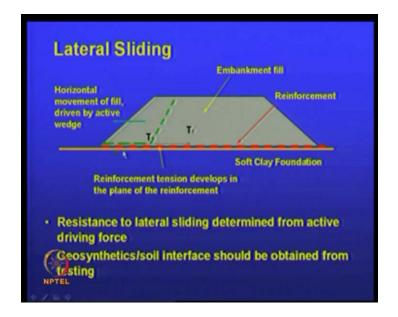
So, that is one way of handling the overall stability, then what is this lateral sliding? As I just mentioned, the movement you address the overall stability, then you need to address this also.
