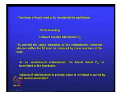
So, if you want to analyze that you have to see this; see, what is a vertical load that we have? And what is an outward shear stress that is coming from this fill? So, to prevent the lateral spreading of the embankment, the horizontal stresses within the fill must be balanced by shear reactions at the base.
