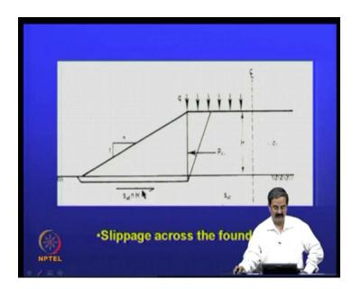
That actually again, here what we do is that. This is a slippage across the foundation right. So, we say, shear strength of the soil into n H will be the resisting forces, and active force is this; which is nothing but you calculate it from gamma H square by 2 into K a into that surcharge and all that.
