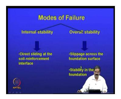
See, because we have placed, why is it the internal stability important? As I just mentioned, you are placing reinforcement, and the reinforcement should not lead to any difficulty or failure.
