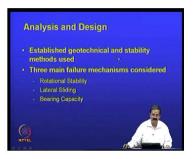
So, what are the mechanisms that we can see here, and we always used established geotechnical methods in this case, and there are three mechanisms that we should address: one is called rotational stability, the second one is called lateral sliding, the third one is called bearing capacity.
