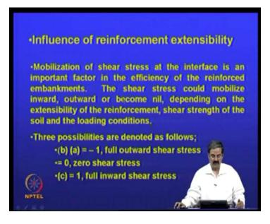
So, how is that reinforcement is helping here? As I just mentioned, the mobilization of shear stress at the interface is an important factor in the efficiency of the reinforced embankments, the shear stress could mobilize inward, outward are become nil depending on the extensibility of reinforcement, shear strength of the soil and a loading conditions.
