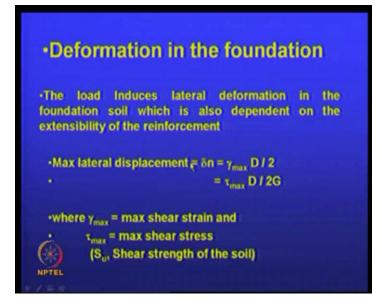
So, that is one thing; so, it is all direct simple mechanics and how do you calculate the deformation in the foundation; like you know the thing is that when you apply load, how much of shear strain it comes.
