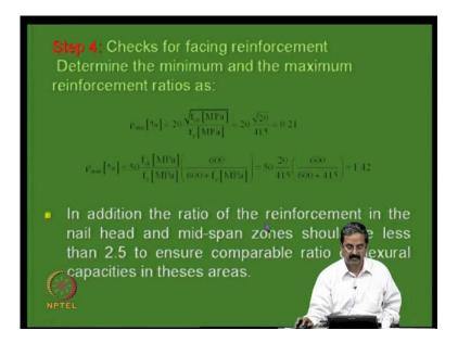
And bearing plate is another one that we provide. So, what we do is that checks for facing reinforcement; the minimum steel reinforcement is provided it is in terms of 20 into square root of f c k into f y 0.21. So, this is another one that we provide like in terms of the. So, maximum value it is minimum and in maximum. It is say the reinforcement ratio it is 1.42 it varies from 1.42 to 0.21 again. So, these are the two expressions.
