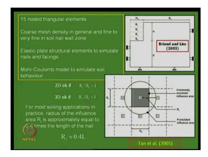
So, this is what an example here is. So, fifteen nodded some sort of examples we have taken and you know the effect which is a fifteen nodded triangular element and Mohr-coulomb model is used and soil soil is a Mohr coulomb model and there is some criteria for the simulation of nails as well all that we have used.
