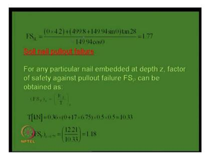
And the sliding factor of safety is 1.77 that all that then the soil pullout nail pullout failure at any depth you have to see that and this is the expression for factor of safety and T N is nothing, but, this expression we have that, k a into the time 10.33 with factor safety it say for example, at 0.75 meters depth level is then given by this expression 1.1.
