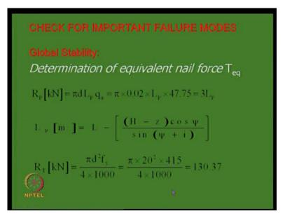
Now, the resistance against pullout is what you calculate and L p you calculate and at any point and this is another thing R T resistance due to tension is what you have provided 130 because it is another force that you 131 kilo Newtons is there in each you know, 20 mm rod that is what it means.
