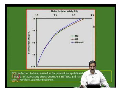
And the thing is that the as a function of construction stage, what happens with different models was seen in terms of the global factor of safety. Like as you saw that the factor of safety is like little higher like three point eight and then it comes down to one point five or whatever right when the construction is complete as a factor of safety somewhat in this range. And there is not much difference between the models used when you are trying to calculate factor of safety global.
