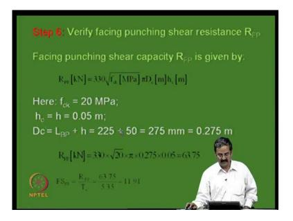
Then punching failure is again there is an expression, simple expression for punching which they have done based on mechanics conservations and here also again same thing you will get 11.91. So, the flexural stability of temporary facing is all right because the factors of safety are quite high and you are essentially using these two expressions here; one is this one and the previous one another thing I showed.
