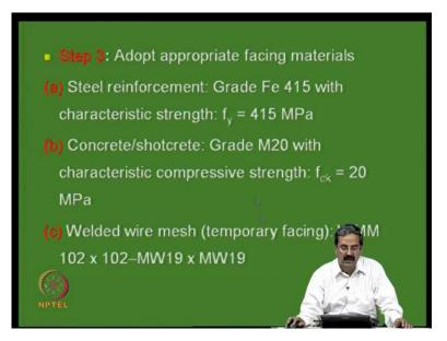
And you know f y grade and m concrete and all that FCKwire, wire mesh you know the thing is that we put a wire mesh. See the thing is shotcreting first thing is the nails are there nails are there, weld mesh is there which is say for example, one naught two into one naught 2 into 19 mm thickness you know some gauge wire mesh. So, there if you weld it and then shotcreting is done. So, that is what we do in our all structures and many places it is done like that.
