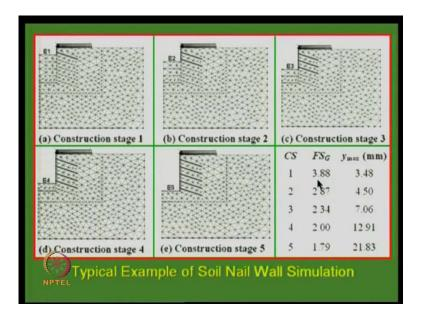
But the best way is to like as I said, the effect of this nailing can be obtained, understood better in terms of finite element analysis. So, what I did was that we did a sort of finite element analysis like typical example what we do is that excavations like I told you know in the beginning like excavations e one, excavation e two there are the different stages you know, e 1 e 2 e 3 e 4 like that you know you just remove that.
