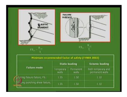
So, one should see that tensile failure and the breakage should not occur. Then the other one is that the what you call the flexural modes you know the facing failure modes right. Failure modes are nothing, but, this you know this sort of plastic movement formations you know, if it is too thin it is possibility to have and even this sort of punching mechanism can occur you know. That is one possibility in the case of facing failures you know.
