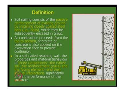
The soil nailing consist of passive reinforcement of existing ground by installing closely spaced steel bars which may be subsequently encased in grout. What we do is that, we sequentially you know make a cut make some little bit of excavation, put a nail you know. It can be a nail means reinforcement bar and it has some, what you call the passive
