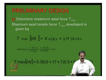
And the maximum force is given in terms of the k a into this particular factors. this is the so, you can see that it is 10.71 kilo Newtons is the force required for this spacing right at a maximum spacing maximum depth of the, you know it is a small number.
