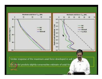
And another important thing that I would like to highlight to you is that you have a tendency to calculate using k a gamma z into s v into s H right. How you calculate the tensile force? Use this expression and then get tensile force. So, if you plot like this, this is a line you get right. Then the thing is that this is from the depth of excavation. So,
