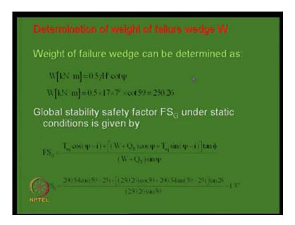
So, this is what we have done. I mean it is double of that actually there is no problem. Now, the weight of the failure wedge is 0.5 into gamma H square cot psi. All these numbers are given. Global stability factor you have an expression here. So, use all of that equivalent tensile force and all that variables, you get a global factors of safety of 1.37 which is okay.
