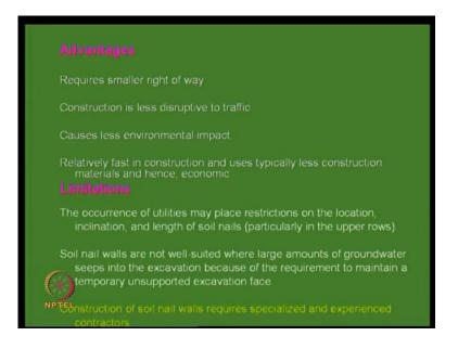
What are the advantages? It is so effective that it can be used you know with some space availability is quite less, construction is less disruptive to traffic, causes less environmental impact, relatively fast in construction uses a typically less construction materials and hence economical then occurrence of utilities may place restrictions on the location, inclination, length of the nails.
