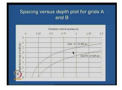
What it means is that, you can see here that if you just plot the grids, the spacing versus the depth plot, this is something very useful to see, at what level the geogrid A will be working? And, what at what level geogrid B will be useful? Like, say for example, if I
