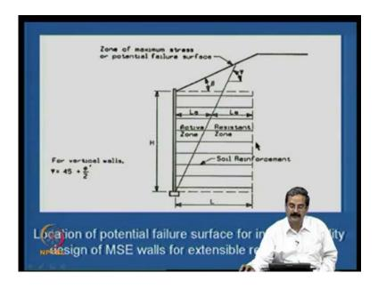
And when you have extensible reinforcement, you have a line like this, which is like 45 minus 5 by 2 line, beta is different. So, in in in this case, it is just the H, and the zone of in the previous case, the zone of maximum tension is like this, in this case like this.
