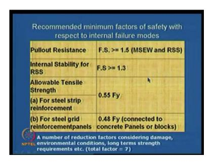
So, internal stability also, like pullout resistance the factor of safety should be minimum 1.5, internal stability for reinforced slopes about 1.3, allowable tensile strength, you know, allowable tensile strength of all these materials is something very high, you know, is it not? Like we have, we know the yield stress of the steel and geogrids or whatever.
