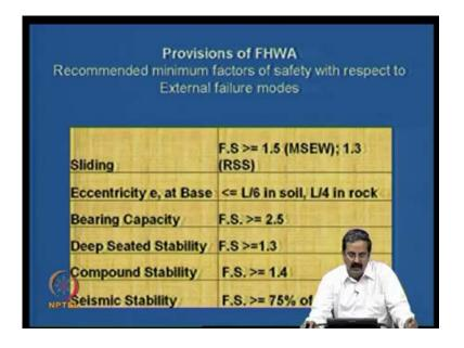
So, some some more information that you know, like we already saw it with reference to the example, what should be the factors of safety? Here, with respect to MSEW means, Mechanically Stabilized Earth Walls; this is a standard terminology that they use, the factor of safety has to be more than 1.5, and then 1.3 in the case of reinforced soil slopes.
