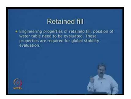
So, this is about reinforced soil wall fill; but there is some material that is next to the retaining wall, which is called retained fill you know; so that retained fill, you know next to that if it is weak, then again there is a problem; you know, whole material should collapse, it it can collapse right.
