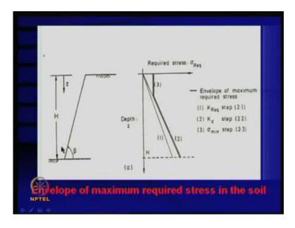
What I want to show you is that this is what I have meant. This is the force, this is actually the reinforcement slope at an angle beta and this one is, that if I just take it as K a gamma H, it will be like this K required, you know, this is, it will be like this, is it not?
