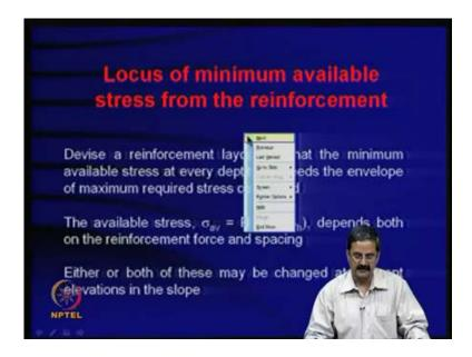
So, we normally try to come out with some sort of reinforcement at the locus of minimum available stress. From the reinforcement we try to device the reinforcement layout, so that the minimum available stress at every depth exceeds the envelope of maximum required stress.
