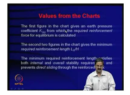
So, the 1st figure in the chart that I just presented gives earth pressure coefficient K required, which is the required reinforcement force for equilibrium to be calculated. The 2nd two figures in the chart give the minimum required length L R by H. The minimum required reinforcement to satisfy both internal and overall stability requirements and prevents direct sliding through the reinforcement block.
