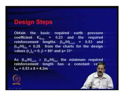
So, what are you trying to do is that. So, I will show you how do you go about this design. Obtain the basic required earth pressure coefficient 0.23 and the required reinforcement length, you know, I just showed you the previous diagram, like you know, that chart. Based on the 80 degrees inclination and friction angle of the, this thing, you will get this required.
