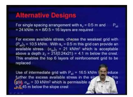
Now, suppose, you are going for a single reinforcement layer throughout that 8 meters level, the allowable 24 by 24 is that and then 0.5, you have 16 layers right at every 0.5 meters. Actually, the thickness, why is it 0.5? In fact, as I just mentioned in the compaction class, that the density within this 0.5 should be same and constant and it should be very good strength and also, it could, it should give very good resistance between the soil and reinforcement, this is very important.
