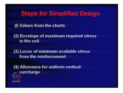
In, in the form of the simple example you have for us, to help values from the charts. You need to construct what is the maximum required stress in the soil, like you know, what is the, say for example, you know, the thing is K, K a gamma H will, will be the stress at any point, is it not? You, if you, you can, as that, that is called the line envelope or line of maximum required stress of the soil.
