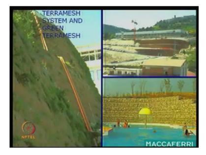
There were many design issues and this is another example that one can have here. See, this is the reinforced soil slope; it could be about 70 degrees. It could, this you can see, that this is also about very high slope, it is not easy.
