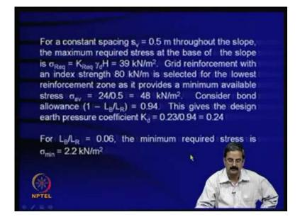
So, now, what we do is that we provide some spacing of those materials for a constant spacing of S v equal to 0.5 meters. Throughout the slope the maximum required stress at the base of the slope is like, you know, k required is what? Point, you have already got the number, K required is some 0.23 and H and all that you get 0.39 you get at the bottom.
