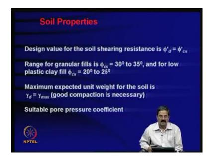
Then, you know, these are all some soil properties and all that, you know how do you like see the moment you want to design the slope you need soil properties. What type of soil is there? So, design value for the soil shearing resistance is nothing but phi by d is nothing but phi dash c s, which value of phi I should take, is it a peak value? Is it a long
