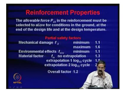
The allowable force P allowable in the reinforcement must be selected to allow for conditions in the ground at the end of the design life and the design temperature.
