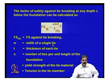
Then, now you have calculated, what is the tensile force you have that is fine. Say for example, it can be you take a meter length of geo textile or any piece of paper, you know any material that you take geo textile, geo grid or something per meter, it has a 10 kilo Newton or 20 kilo Newton or 50 kilo Newton or whatever; even steel may have higher reinforced high tensile force carrying capacity.
