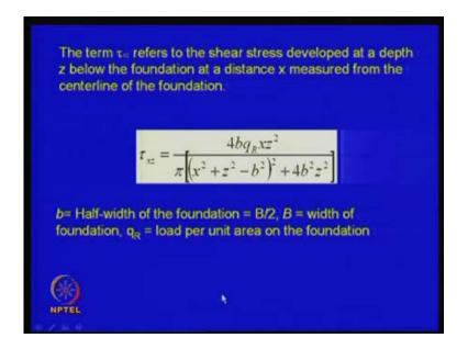
As I just mentioned, the elastic shear stress distribution is used. This is the expression that we have in theoretical soil mechanics. And if we know the x and z and b is nothing but, the half width of the foundation; q R is the load that you are expecting you know that is the reinforced soil load. Once you have this and then you can plot this, it is simple.
