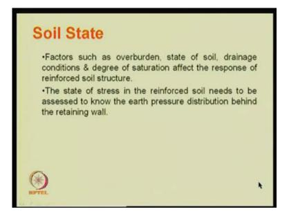
Then, the soil state, see there are number of reasons here; one is, say we said, the we said cohesive soil is also ok and then we also said sand is fine, but then soil alone is not sufficient; soil state, what is the state of the soil and how does it respond. So, for example, at pull out over burden, you know, so for example, in a retaining wall, you have 1 meter, 2 meters, 3 meters, there 3 or 4 depth of over burden is there you know or in an excavation depth of over burden is there.
