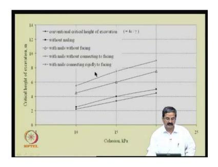
This is again same thing, like if you do connection, what happens? When you do with connections, what I just observed was that, it will be having higher critical depth of excavation, which means that, the forces are little transfer to that. And also actually we have seen that, the failures surface the shifts towards the facing and the mass of the soil, that creates earth pressure is going to be less.
