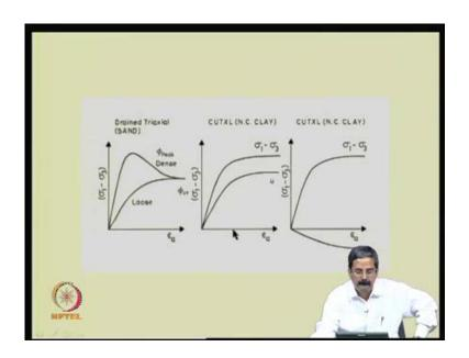
So, these are all some typical stress strain curves that we see in the case of test. So, this is in the case of peak, we have a similar response here, like essentially this is a pore pressure response; and this is in the case of drain test, this is a volume change, ok.
