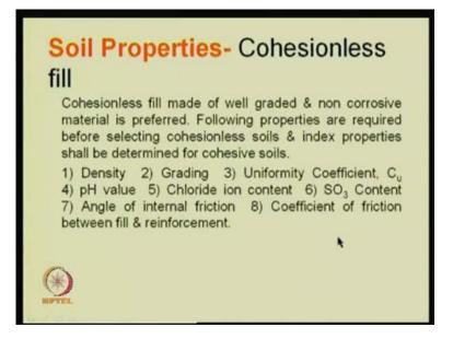
And see the normally in codes, we specify well graded non corrosive material, and we need to have the following properties like density gradation, uniform coefficient, ph value, chloride ion content and all that properties are required, and coefficient of friction between the soil and reinforcement are required.
