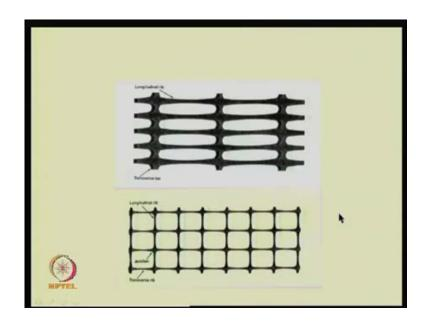
It can be like as I just mentioned, it can be a geogrid. This is most of the time we use it for reinforced slope applications or retaining wall applications. This was used for bearing capacity and pavement applications, like say the thing as I just mentioned here, this is a geogrid and these are direction of axial force, and there is a contribution of grid.
