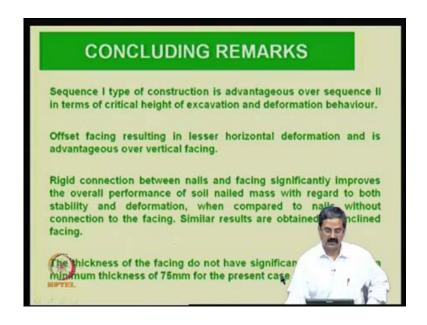
So, what I would like to just summarize is that, effect of sequence is very important and these are all some observations that we saw. Rigid connection between nails and facing improve the stability of the soil mass, both in terms of factors of safety or even deformation and all that.
