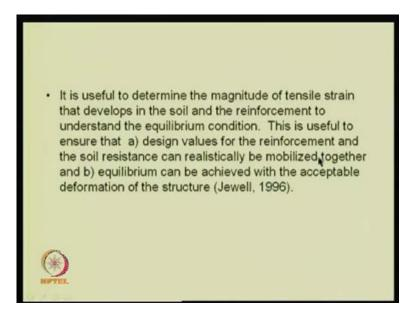
Why this is very important, because it is very useful to determine the magnitude of the tensile strain that develops in the soil and the reinforcement to understand the equilibrium condition. This is useful to ensure that the design values for the reinforcement and the soil resistance can be realistically mobilized together, and equilibrium can be achieved with the acceptable level of deformation of the structure.
