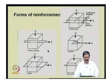
So, forms of reinforcement as I said, it can be a strip, it can be a sheet, it can be a grid, like I will just show you; there it can be a anchor, like you know, you have a reinforcement, you can put an anchor inside; you can be a just a simple bar like a reinforcement bar.
