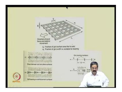
There are two things here; the interaction takes place between the soil to soil, like you know, here say shear between the soil on plane surface, like you know, here you have. Then, you have bearing also like this, like you can see that, you know when you pull a
