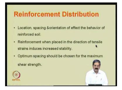
So, reinforcement distribution is another important factor. We have seen that, say for example, if there is a load applied on the footing and failure planes develop like this, so you put reinforcement in the horizontal direction. So, the possibility is that, the reinforcement will intersect the shear planes and then it increases the bearing capacity.
