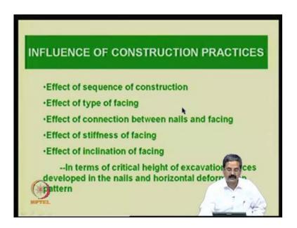
So, once you have these sort of information, one can understand as I said construction practice how is that it is influencing here. So, sequence of construction, type of phasing, connection between nails and phasing, stiffness of the phasing, inclination of the phasing also, we will just see that.
