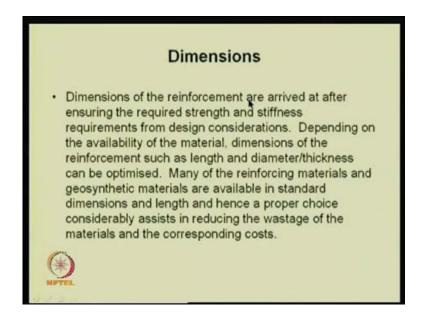
Then, dimensions actually, you know, the way that we design is that, we just first get some required strength and stiffness from design, and say we try to check, if it is available; say for example, tensile strength is a 30 kilonewton per meter and we should know what length it is available, because I need if 7 meters is a height of retaining, say for example, 10 meters is the height of the retaining wall, 0.7 times is the length of the reinforcement required.
