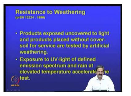
So, you can find out its corresponding property and do that. So, resistance to weathering: what is that, it is essentially that, the products exposed to uncovered light, you know, if you do not cover them properly, the possibility is that they are exposed to ultraviolet rays; and the possibility is that, it gets... see the thing is, you just leave, you know, I have seen you just take a geosynthetic material and leave it outside.
