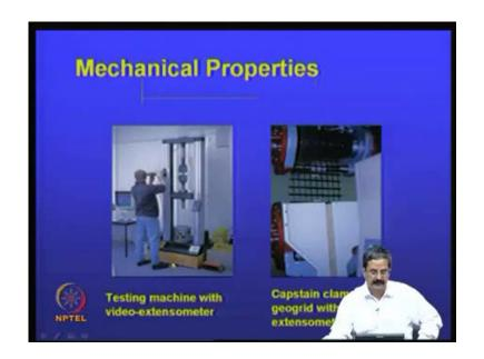
Mechanical properties you can see that, see this is a material that is being tested; here is a geogrid or a geotextile here. So, testing machine with video extensometer like, you know, they see that deformation in the on the strain using sophisticated equipment, such as video extensometer. Here, they are trying to use laser extensometer; you have a geogrid here, you can see that, it is being pulled up and they are trying to measure that strain.
