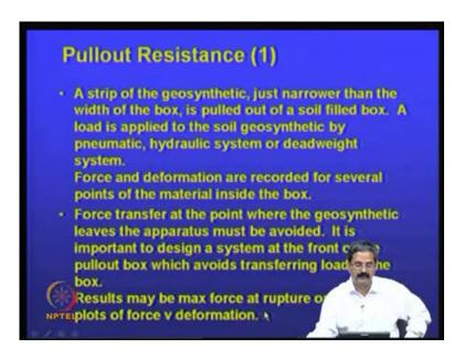
So, you can see that a typical result corresponding to a 50 mm, right, is taken as the angle of you know friction angle. This is another test which we have to do is called pullout test. Actually, as I just mentioned the concept of reinforced soil, you have a friction in the
