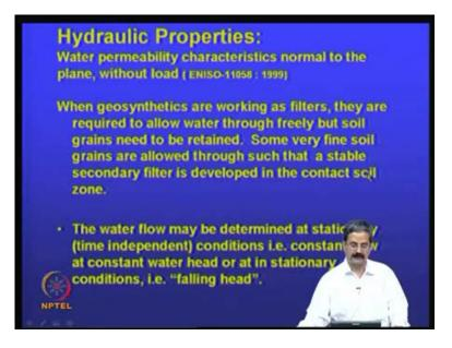
So, again we have a lot of testing procedures. When geosynthetics are working as filters, they are required to allow water through freely, but not the soil grains. So, sometimes some very fine grains are allowed through, such that a stable secondary filter is
