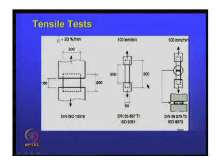
So, these are all different standards as I just mentioned. And then, there is a rate of application of load is also mentioned; 100 mm per minute, and so, this is like, say, in this case, it is a 20 percent per minute, like this they have some. So, these are sample size, here as I just mentioned, these are all sample sizes.
