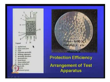
So, seven is the geomembrane, then you have a geotextile; this is actually the aggregate. Actually, see, we normally use in the landfill, aggregate as a... even in a payment also, we are using aggregate as a drainage medium, so but then the drainage medium should not puncture the geomembrane.
