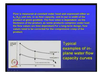
So, flow is measured at constant water head and expressed either as permeability in meters, or the flow capacity per unit width, like you know, per width at a given hydraulic gradient. So, for different hydraulic gradients, we can get this material. So, the flow is
