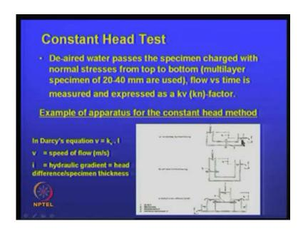
So, there are some tests here, unlike what we studied; you can see that, this is a geotextile material; it is not a similar type that we know and soils. So, de-aired water passes through the charged specimen with norm; so, it comes like this and then you measure this, and this is what is called for the horizontal permeability, where geotextile
