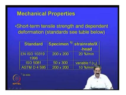
In fact, short term tensile strength means immediate tensile strength and you have certain standards for it, and this a specimen size is at 200 mm by 200 mm, this is a size and then the strain is given also. These are all actually, you have European standards, you have I S O standards, you have ASTM standards, all these three things are very important, because if you are in Europe, you may try to follow it; ISO is a general standard, ASTM if you are in US, they you know go by ASTM standards.
