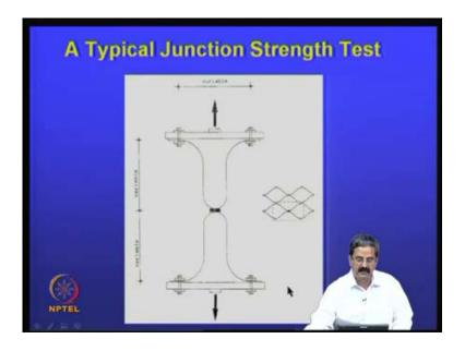
So, we try to test them for a typical junction strength; see for example, this is what I mentioned, was a geocell. So, this is what is called junction strength. So, if that is not good, then it is not going to very effective. So, you have to test this particular junction strength. So, you try to calculate that here using some the procedure.
