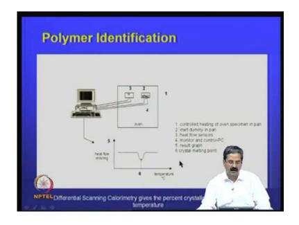
In fact, if you want to identify the polymers, there is a test what is called differential scanning calorimetry; when which you have a sample here, then you heat, you know, you have a sort of a control heating, and then once you heat rise the temperature, there is a what is called heat flow is monitored as a function of the temperature.
