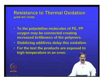
Then, resistance to oxidation as I just mentioned, to the polyolefine molecules of polyethylene, polypropylene, oxygen may be connected creating increased brittleness of the polymers. As I said, brittleness is one thing that can, you know, because of the
