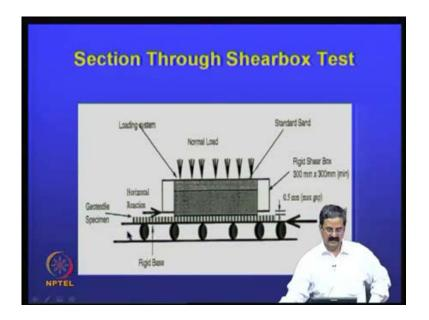
And this is like this, you know, direct shear test we are familiar; and what we do is, that here it is one thing very important is that, see the our direct shear test whatever we have needs a bit of modification, because you must be able to in direct shear, we do a normally a sample here, you need to do a for a big sample, say not less than one foot by one foot or something like that, which represents the actual field condition.
