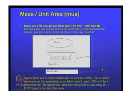
We also need to know it is a mass per unit area, which is called we know mua and it is one of the very important applications here again. And you try to take a small circular piece of geosynthetic material and then weight; so, you take its weight. And In fact, as I just mentioned, the quality of a paper and the quality of silk is also measured in terms mass per unit area.
