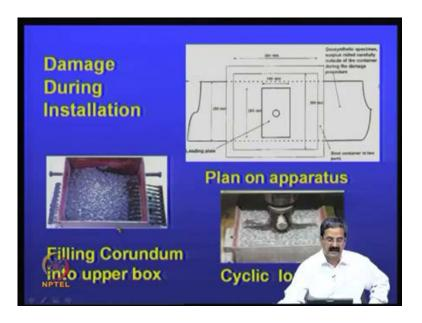
So, this is, say for example, this is like this. Damage during installation, filling up in this corundum box, this is that a geogrid material, and cyclic loading is applied and this is all geosynthetic specimen; surplus is rolled carefully outside this container during the damage procedure. So, these are all some sort of testing that is done.
