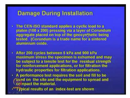
And there is another test what is called, you know, if you want to understand what is a damage that can occur during installation. Again, this is an European standard, in which you have a cyclic loads applied 200 cycles between 5 to 900 k P a and maximum stress is assumed. And so, after the maximum stress, the specimen removed and again you test it for tensile test or a filtration test.
