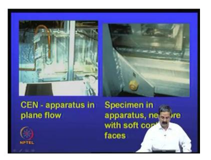
So, this is the type of test, for the in-plane flow test; this is a specimen in apparatus, net core with soft contacts. If this that you can see that very clearly, that geocomposite net core **net**, geonet is nothing but a drainage material. So, they have placed that material here and then they are testing it; this is a very important thing.
