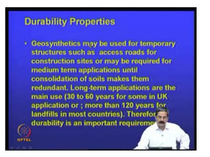
So, you need to see resistance to weathering, resistance to microbial degradation, resistance to liquids, resistance to hydrolysis, the resistance to thermal oxidation. So, actually geosynthetics may be used for temporary structures such as access roads for construction sites or may be required for medium term applications, until consolidation of soil takes place and redundant.
