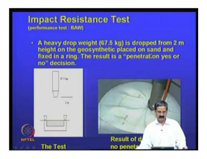
This is how it is done, like, as I just mentioned a small, drop weight, lead platen, specimen under ring. And this is what it does, you know, you can see that , this is impact resistance test, this is standard test actually. This is how it is done layout and this how you know after that this another same type. And the result is, penetration yes or no, that is what it is shows; and if there is no penetration, it is suppose to be good like that.
