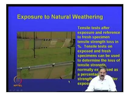
Then, there is a what is called exposure to weathering. Tensile tests after exposure and reference to fresh specimen tensile strength loss is there, like you know, you expose it to different tensile testing I mean different degrees of weathering here, like keep the samples for 1 year 6 months, I mean, like normally say for example, a phd program definitely that person can test for two and half years, like immediately as soon as it registers take the fees and then put it like this like.
