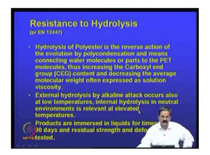
So, this hydrolysis is again is something, that hydrolysis of a polyester is the reverse action of the evolution of polycondensation and means connecting the water molecules or parts to the PET molecules, thus increasing the carboxyl end content, and decreasing the average molecular weight often expressed as solution viscosity.
