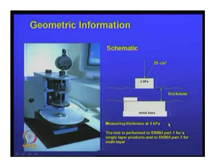
The geometric application, actually the thickness is quite important, because we have seen varieties of materials, they have different thicknesses. And as I just mentioned, we have to standardize at one pressure, at 2 k P a, we measure the thickness; actually this is a thickness of the sample, this is a weight and area of cross section is there.
