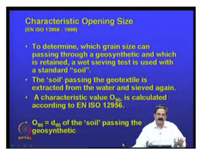
As I just mentioned the apparent opening size or the size of the geotextile is another important parameter, like, see, we know, we we design the filters based on gradation size, we say d 60 size d 10 size d 30 size and all that.
