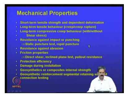
Mechanical properties is what we need in most of the applications. So, we are looking at short term tensile strength and corresponding deformation; long term tensile behavior, like, it can be in terms of the long term means; the time dependency like, you know, you just wait for different periods of time and then find out, if what is a change in tensile strength.
