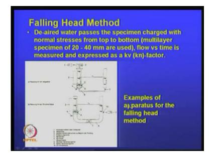
So, it can be even for, you know, from flow versus time is measured. And you have that, using the Darcy's law, one can calculate the permeability; then falling ahead again similar thing was done. Here, again a de-aired water you know, in fact, in permeability testing we should used de-aired water, because you do not want air in the water.
