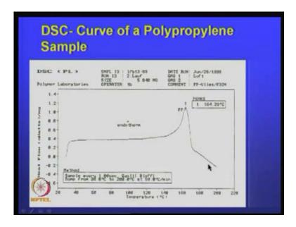
Then, the crystal melting point is somewhere here; it is a function of the type of polymer you have; and so, that can be used as a basis to identify the type of polymer. So, for example, here, you have the polypropylene product, you have a about 164 degrees, 0.29 degree centigrade, you have this type of result you get and people can use some of these materials for whatever is the application that we are interested in.
