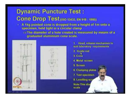
You have a dynamic puncture test in which a cone is dropped from a height, about a one kg pointed is dropped from the height of about a 1 meter onto a specimen, held tightly in a circular clamp. The diameter of the hole created is measured by means of a graduated aluminum cone scale.
