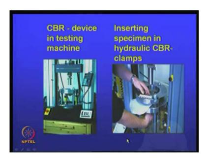
And resistance to static puncture: actually, this is actually a modification of the CBR test, because what we do is that, here we try to use this test for, you know, things like this; you know CBR test, we try to make a puncture here, means, you know, we try to measure the load here; essentially we try to say, similar to the C B R test, we measure the load versus deformation; here also we get the same thing.
