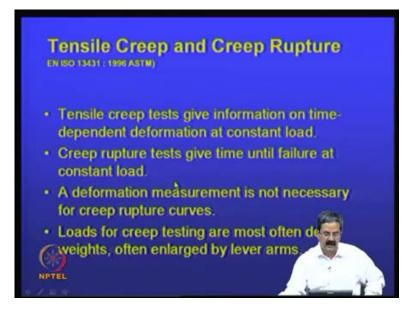
And the other important properties called tensile creep, like, you are doing a tensile testing, but then you allow apply the same load, but still there is a creep, you know, like, if there is a load that is applied. So, the tensile creep is an important parameter; it gives information on the time dependent deformation at constant load.
