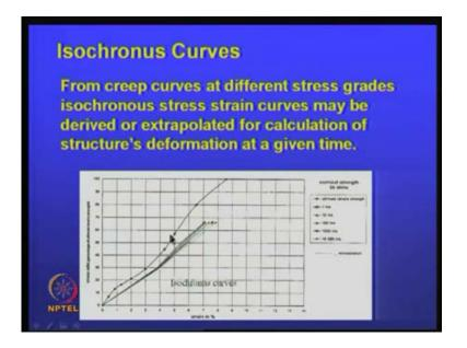
And so, creep rupture is one possibility; this is the way that we construct creep load curves. And from this, we construct what we called isochronous curves, which means that, at the same time, we would like to see what is its effect of, say for example, here the tensile strength of that geogrid is or geotextile material is 35 kilonewton per meter.
