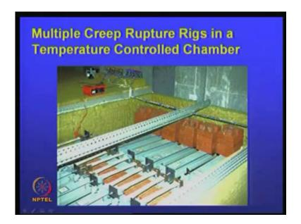
And multiple creep rupture rigs in a temperature controlled chamber, in fact, in a chamber where you have multiple materials tests are being done, and all that this is one.
