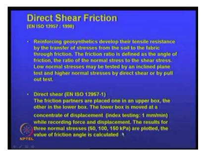
Then, there is another one what is called direct shear friction. Here, the direct shear friction is something that is very important, because as I just mentioned, it is the reinforcement reinforced soil is essentially because, you know, there is a friction between the soil and reinforcement, and that friction is converted as a tensile force.
