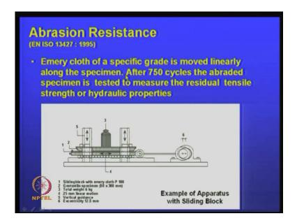
There is another test called abrasion resistance test, like emery cloth of the specific grade is moved linearly along the specimen. After 750 cycles, the abraded specimen is tested to measure the residual tensile strength or hydraulic properties.
