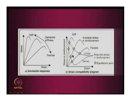
What we need to see, is how both reinforced soil as well as how the reinforced soil behaves; and as I was just mentioned, we have different types of reinforcement elements. One is called, one can be a steel reinforcement; in the case of, like, you know, steel reinforcement, like a geo-grid, like a steel grid, you know; it is very stiff stressing properties are very good, you know; stiffness is there.
