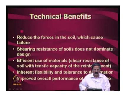
Why is it, the technique has been effective? Actually, the thing is that, we should see, why the reinforce soil is effective, and from technical angle and as well as economic angle. In terms of the technical advantages, see, if there is a force like it reduces forces in the soil, which cause failure like, you know, there is a disturbing force and earthquake force in the opposite direction, which means, that it reduces the forces in the soil, which causes failure.
