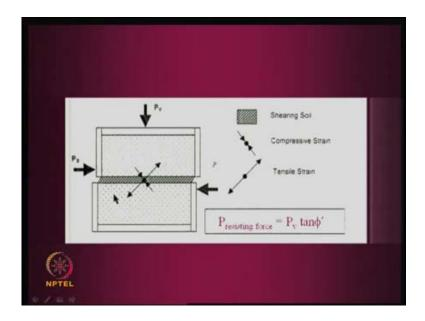
So, how does it act? We have to see and quantify, we will see that. See, this is analogous to a direction of box, you apply some vertical force, there is a shear force, right? And, what happens? This is a soil without reinforcement; and in this soil element, which is under sheared, there is a compressive force like, you know, because of this movement, in this direction, there is a, you know, its compressed in one sense like.
