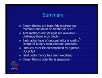
So, what I want to say is that, this Geosynthetics are bonafide engineering materials, and must be treated as such; you have testing methods and designs that are available. And the
