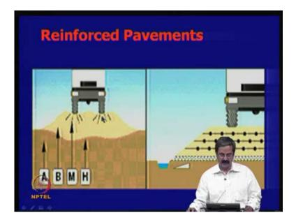
You can see that the area of cross sections, so much could be saved in the case of pavements; that is what I was telling. That it is possible to have rutting failures as well as, rutting failure means deformation failures and as well as fatigue failures, which are because of the repeated application of loads. Both can be seen that you have a higher resistance with this geogrid material; and you also have a drainage here, you can just
