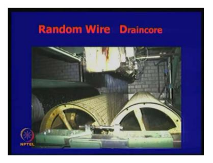
Like, again random drain core, you know. Say for example, as I just mentioned of our pre-fabricated vertical drains, we need to have drainage core, you know; like we have a geotextile as well as a geofilter.
