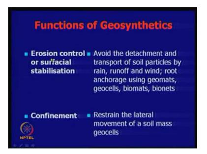
Then, another important thing is what is called Confinement. The Reinforcement also provides some sort of confinement. Nowadays, you have a geocells which are very good, which can provide good confinement.
