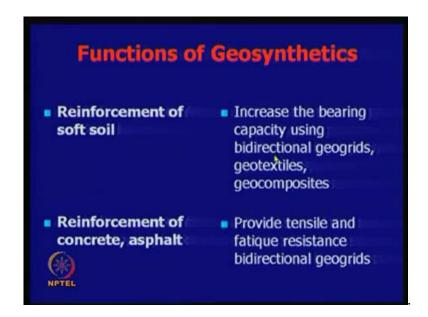
So, Reinforcement of soft soil: it increases the bearing capacities in bi-directional geogrids, which are like this, or even it can be like this; where you have a bi-directional geogrid can be used, this also can be used. It is called some product secure grid, which is a quite a very good material.
