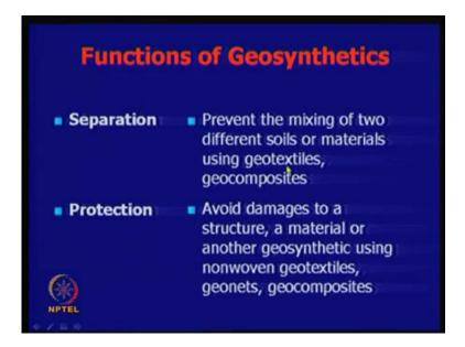
You can do this by any material which can be used for separation; essentially, geotextile is used, because it is much cheaper and prevents the mixing of both the materials.
