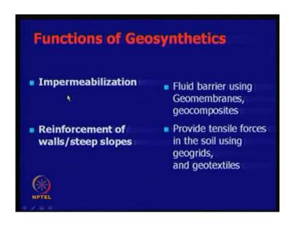
Then, very important thing is Reinforcement of walls and slopes. This is actually, of course, it provides tensile forces in soil using geogrids and geotextiles. Of course, this is a bi-oriented geogrid, and we will see in some of them, mono-oriented is also possible
