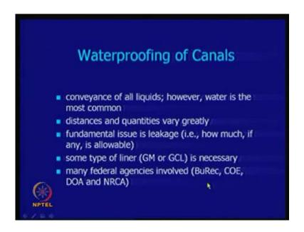
Then, water proofing of canals. Actually, in many of the places in India, at least we have we have what you call in many of the water supply and for irrigation and all that, for drinking and all, for particularly irrigation canals instead of the canals. And they have lot of quantities going through them; and, if there is a problem of seepage, then it is very significant. Like, you know, say for example, if 20 to 30 percent is through the leakage, then it is going to be very risky.
