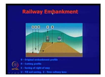
This is another example where, in the case of railway embankments, the earth ore can be saved. If you are able to construct the slope in this manner, using the RU wall, reinforced earth soil technique, reinforced soil technique, you are able to save this much of soil; and it is going to be much more stable as well. So, essentially, you can design some of these things in a very comfortable way; this is in a highway embankment.
