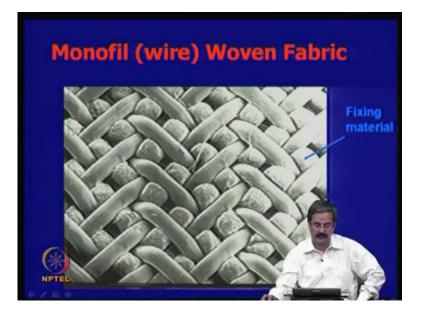
This is monofilament like, you know, single filaments, and they are all woven together. So, that is about geotextiles.
