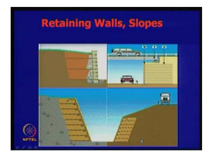
These are all some examples that we will see where... See, this is for the reinforced earth wall; you have a layer of geo; see, this is a backfill; this is a, this is actually we call it a backfill. This is a wall fill; wall fill means, the wall, the fill that is next to the wall. Then,
