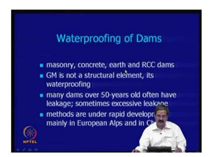
So, in the case of water proofing, like normally masonry, concrete and earth dams are used; and so, for which if you want to have water proofing, you need to have good geomembrane. So, it is, it is for water proofing that we provide. And particularly, there are many dams which are old like, say for example, fifty years, they have lot of leakage and sometimes excessive leakage.
