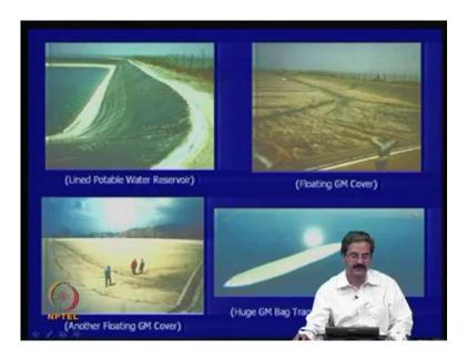
Say for example, this is potable water, which is stored. And then, the potable water should not be a leaking; so, you need to have a geomembrane, geomembrane for that. Then, see, the thing is that you should be very careful; as I just mentioned earlier, the friction between the soil and geomembrane, geomembrane could be very low. So, it leads to some sort of a, you know, it floats like if there is no, like, if there is because of slightest pressure, it can get lifted up.
