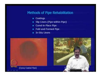
So, what we do is that, we try to line them with some; you have coatings, you have slip liners, you have curing in place and there are in-situ liners, like this pipe within pipe. So, there are so many techniques that one have, one can have. And so, now, I would like to show, how these materials like fibers and tapes are all made.
