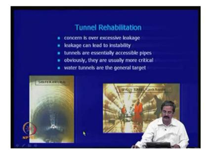
Even in some places, you know, tunnel rehabilitation like, you know; say for example, in some places, you cannot use the tunnels because of the excessive leakage, and leakage also leads to instability. So, then, what we do is that, this sort of, see this is a typical case; then they try to put a layer of geomembrane, geomembrane and all that. There is a systematic design here; so, these tunnels are whether it is for the water supply or for whatever purpose we have, we can rehabilitate.
