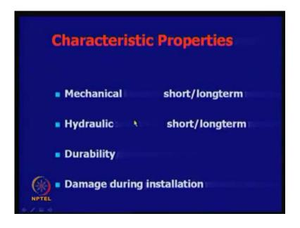
Some important characteristics one should remember was that, you need to have some mechanical properties, understanding them. You should also understand that, say for example, mechanical properties means strength and stiffness. Strength is nothing but, you know, as I just mentioned, that the ultimate tensile strength. Say for example, you
