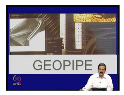
The other one is what is called geopipe, actually in many of the land fill applications. We are using, you know, all the leachate has to come out of the pipes; even our water supply pipes, we do not call them geopipes, why? But then, this term has become very important, because when you are using in the olden days, people were using concrete pipes, where the soil next to the concrete pipe does not have any role to play.
