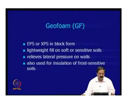
It is like a it is foamy material, it is a very light weight fill on soft and sensitive soils, relieves lateral pressure on walls. It is also used for insulation of frost-sensitive soils; actually its another very important material in fact its compressibility is quite low. But at the same time, its easy to lift, like we have seen that two people have taking it, carrying it.
