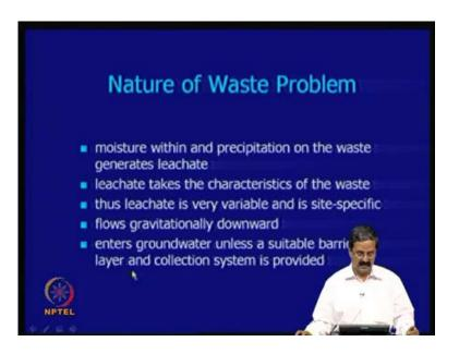
So, for that, you have a secondary linear systems in the field; that is how it is installed and you have leak a geonet leak detection systems, like you know. In fact, you will have lot of sensors in the field; in fact, I will show you some photos, where they will measure in the particular landfill like this, because of the rain, how much of leachate is generated.
