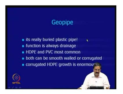
So, it is in fact the geopipe is nothing but a buried plastic pipe; the function is always a drainage of leachate. High density polyethylene and polyvinyl chloride PVC is most common. If you go to lab or even Yashvanthpur anywhere or any place, you know, most commonly PVC pipes are used. Both can be smooth walled or corrugated; corrugated high density growth is enormous; nowadays high density polyethylene pipes are quite popular.
