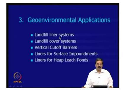
We know that waste is an issue, that everybody has to address and on the waste if the precipitation occurred it generates leachate. Leachate takes characteristics of the waste and the leachate is a highly variable and site specific and the flow is always downwards. And we should see that, the groundwater is not contaminated, because of this leachate travel and you need suitable barrier and a clay leachate collection system.
