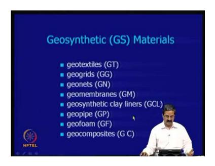
And you have what you call geotextiles, geogrids, geonets, geomembranes, geosynthetics clay liners, geopipes, geofoams and geocomposites; anything that connects ground and improves its performance - ground performance - essentially we are looking for ground performance in terms of the engineering applications.
