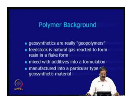
The geosynthetics are essentially geopolymers, in the sense that, they are all polymeric materials. And you know, they are from the natural gas reacted to form resin in a flake form; in the sense that, when you are trying to remove this gas, you know, you have a
