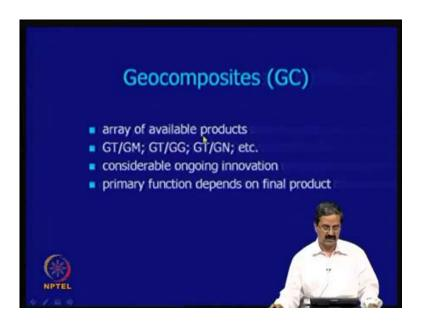
So, geocomposites can be, you know, it can be a geotextiles and geomembrane glued together; geotextile and geogrid you know together, like say for example, geotextile can serve as a drainage material; geogrid can serve as a reinforcement material. So, in this case, geotextile can just act as a filter material or drainage material; geomembrane may not allow all that water to go down.
