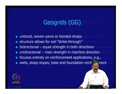
So, the geogrids are something that we have a special type, where the unitized woven yarns or bound straps. Structure allows for soil straight through, in the sense that, there is soil to soil contact as well as soil to grid contacts.
