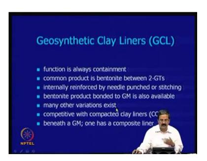
So, the function is that, again their function is always a containment like in the case of a clay liner; clay liners containment, you know, they contain all the waste, ok. So, when clay liners are not effective, better to use clay just with the clay liners, because they are all manufactured products. So, the common product is a bentonite, which is sandwiched between two geotextiles; internally reinforced by needle punch to a stitch bonding.
