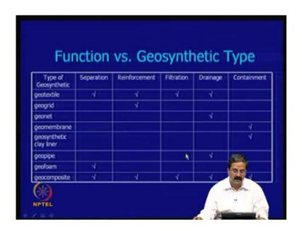
So, I would like to just mention that, they have very good applications, separation, reinforcement, filtration, drainage and containment - their main applications. And geotextile can be used for separation function, and geofoams also can be used for separation function and geocomposite.
