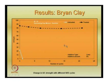
This is another one unconfirmed compression test. Again, see, that it is somewhere here in the case of untreated material the shear strength we use. Actually, it is so poor, that it is a very small value.
