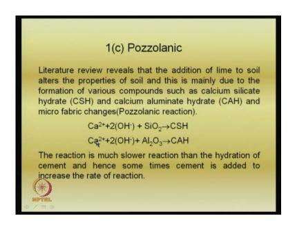
Another important property that we should understand, that lime gives a sort of pozzolanic character to the mixed soil. What it means is that it results in calcium silicate and calcium aluminates hydrate materials and also changes in the fabric changes. So, it leads to two compounds like this and it is like, you know, we understand that the same
