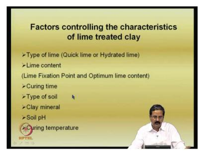
And what are the factors, that influence the characteristics of the lime treated clay? One should be able to understand the characteristics of the lime treated clay and one is the type of lime, whether it is a quick lime or hydrated lime; lime content, like what is the percentage, that you are trying to add; the curing time, say for example, it can be different from one day, 2nd day, one week, one month, one year, it could be different.
