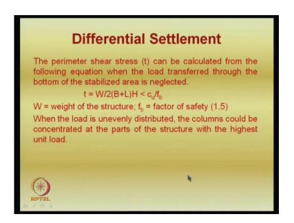
So, the perimeter shear stress can be calculated from the following equation when the load transferred through the bottom of the stabilized area is neglected. So, this is what I just mentioned, like people are (()).
