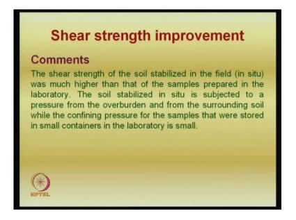
And how is that the strength of the soil is improved? People have seen, that like you have seen just now, that the CBR is nothing, but the strength of this in situ soil and you add lime, the strength of the soil is increased by about 30 times, 40 times, 50 times. In some cases, in situ CBR test was done in some cases, we have seen that.
