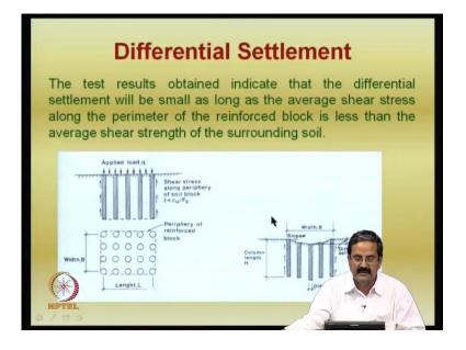
Another important point, that we should give weightage to, that is, that suppose, you are trying to construct a structure here. So, the, you need to calculate the ultimate bearing capacity is one thing, like you know, the thing is, that bearing capacity is one thing, you should also calculate different settlements and total settlements, that is very important, then the design is complete.
