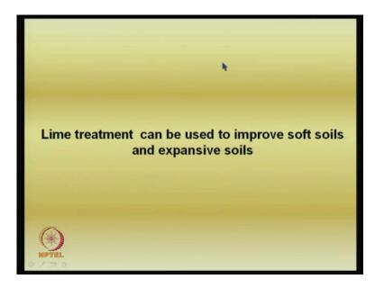
Lime in the ground treatment or ground improvement. The lime treatment is something, that has been quite popular with many of the civil engineers and whenever there is a problem with soft soils and expansive soils, lime treatment has been given and essentially, to improve the bearing capacity and reduce the settlements. We will see how this lime treatment can be effected in the field and what are the various factors that can influence the treatment?
