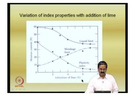
This is a typical example of how the mixture of lime with water can change the plastic characteristics. For example, if you see the liquid limit, it is about 60 percent here with 2 addition of percentage of lime, 2, 4, 6 and 8, you know, liquid limit has come down, some 60 to 40 percent.
