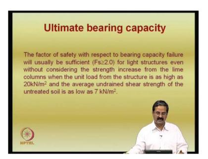
And the how do you get the ultimate bearing capacity? The ultimate bearing capacity is obtained from the strength of the samples, like you know, actually we, you know, for example, unconfirmed compressive test is one simple device, simple test one can do and as I just said, the confirming effects are there, particularly when you are trying to use this.
