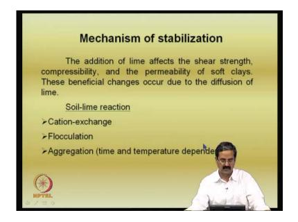
So, what we should see is that, what are the mechanisms? And the, as I just said, the mechanism, it results in improvement of shear strength, compressibility and permeability. So, what are the reasons or mechanisms?
