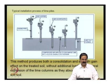
So, how do you do this installation? Say, for example, this is a hopper like, this can be connected to any of the vehicles or something like that, just insert and they have lime aggregates and materials and all that go to the, you have a compressed air arrangement applied to this as lime into the whole, as a casing is withdrawn, the, you are trying to remove the casing and then, the lime is getting added here. And you can complete the whole process and you have the lime column formed.
