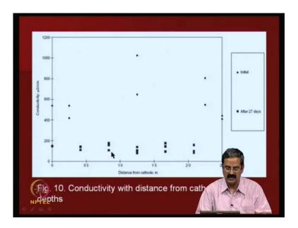
So, the conductivity of a solution is governed by the movement of ions within the solution the factors effecting the solution conductivity or the concentration of the ions, quantity of the ions, the charge of each ion, freedom of the ionic movement, solution temperature and all that.
