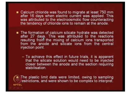
So, in a nut shell what it means is that, it has been quite effective and the formation of calcium silicate hydrated was detected after 27 days. This was attributed to the reactions resulting from the mixing of calcium ions transported from the anode to the cathode. So, this is what they have done.
