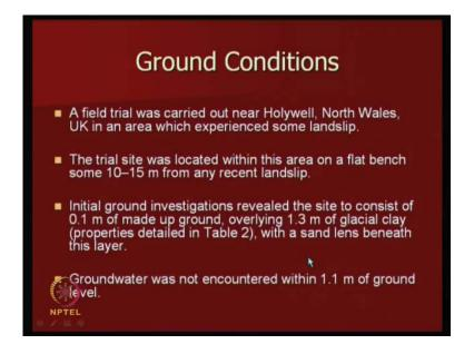
There are very interesting examples. You have a field trail that was conducted in UK and there was some land slip that occurred and close to land slip they constructed this particular field trial. And initial ground investigations revealed that the site have a 0.1 meters of made up ground, overlying 1.3 meters of the glacial clay, with a sand lens beneath the clay layer. There is no ground water within 1.1.
