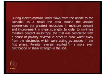
We also talked about P V Ds just now. Here also even you can accelerate the consolidation of P V Ds also using this. And there was an experiment done. And Electroosmosis was then applied for a 500 hours which produce further consolidation of 340 mm and an increase in shear strength from less than to 15 to 30. It is quite excellent. So, they are able to observe some of this, whatever you observed the greatest water reductions in moisture content and the improvement in shear strength.
