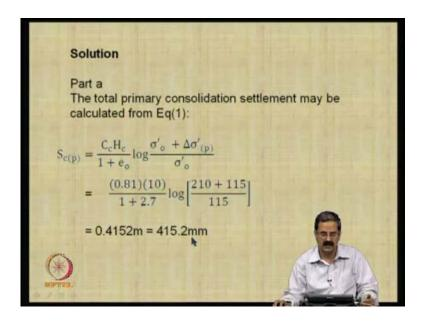
We have seen this in the last class and it is about 415 mm, is a consolidation settlement that you can expect and that with figures like this with the principle that we have studied last class. We can calculate that knowing the degree of consolidation at midplane potential and time factor and all that.
