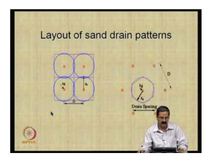
So, we saw that the same example the settlement is about 415 mm and this is a typical patterns that we have seen in the video also it could be triangular it could be square.
