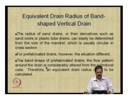
This another important point that one should realize and like the difference is that we had an equivalent diameter there and now since the shape of the sand drain is something you know more of a rectangle the flow pattern around the drain is considerably altered from the cylindrical case.
