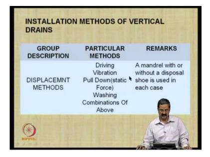
So, how do we install it? there are some typical methods like it can be, you know displacement methods; like it can displace the soil of course, the soil is so soft it can be displaced nicely and particular methods you have vibration; driving vibrations and pull
