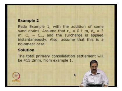
Say for example, I assume I try to deduce the example with sand drains assume that the radius of the sand drain is about 0.1 meters or 10 centimeters diameter; radius or 20 centimeters diameter. And the effective diameter as I just mentioned last time that there is some area of influence around which it acts as a drainage layer. So, you have a sand drain and there is some area around which it can be very effectively considered as a drainage layer.
