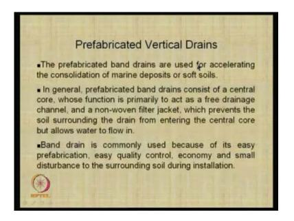
And as I just mentioned, PVD s are much more comfortable to use because of ease of fabrication quality control economy and sample disturbance to soil is very less during installation.
