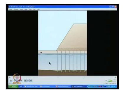
You have an embankment here, you can see that they are very close. Like you know these are all say for example, this could be the heavy embankment of 5 to 10 meters and not about 5 meters you can say that and you can see it once again like a series of prefabricated vertical drains, installed actually in the field. This is that once it is done you have actually you can see a drainage layer; also here, then you have this embankment may be about 4 to 5 meters.
