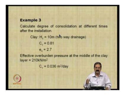
Because we are claiming that or we are, we know that this consolidation you know like it can be very low and then we would like to increase the consolidation using the sand drains or prefabricated vertical drains.
