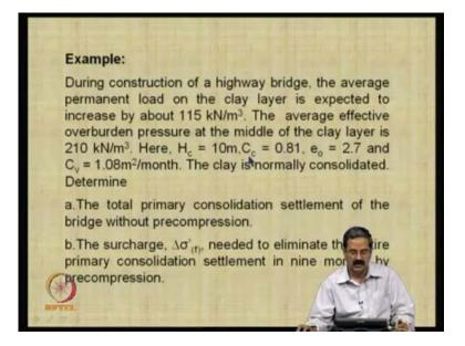
So, as I just mentioned I gave an example last week, last class where you had some sort of surcharge which is because of the pre load; in fact, this 115 no. You assume that there is a permanent load that can come because of the extra load that 115 kilo newton per meter cube. These numbers can be calculated using, you have numbers of theories or elastic solutions where you know the load of load whether it is a uniformly distributed load or point load or even a triangular load.
