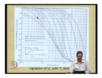
So, and then like I will show you this figure. This is what I was just mentioning that the ramp loading actually like excess pressure that we have applied on the soil ok. So, now this is called the degree of consolidation and then this is the time factor. So, the numbers in the circles are the construction time factors like as I just mentioned we have time construction like in the previous example previous slide; these are the two factors.
