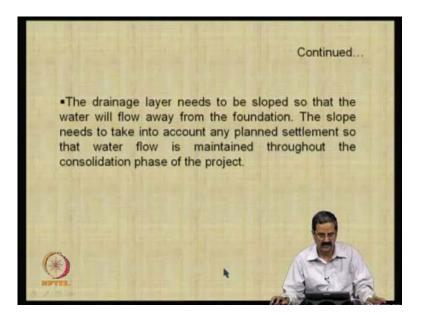
The drainage layer needs to be so sloped that the water will flow away from the foundation area like that is very important the slope needs to take into account any planned settlement. So, that the water flow is maintained throughout the consolidation phase of the project.
