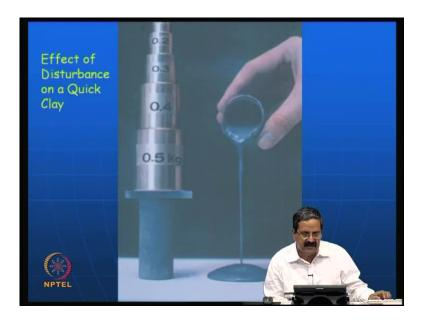
This is another classic case of soft soils. In fact, you can see that the sampling disturbance on the case of undisturbed soil, it is able to take lot of load like you can see 0.5, all that loads you can say an undisturbed sample.
