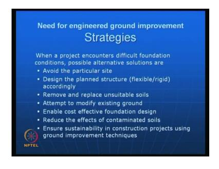
So, when a project encounters difficult foundation conditions like, you are trying to construct a road or a building, what are the solutions. So, you have an expansive soil, are you going to construct a road on an expansive soil? The problem would be that, the moment you construct an expansive soil after two seasons, all the payment is just get curled up and you are treated as a bad engineer, we do not want that.
